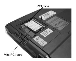
3. Push the **mini PCI slot clips** outward and pull the **mini PCI card** out of the connector on a 45 degree angle.
