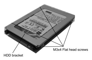
6. Remove **four M3x4 flat head screws** securing the HDD bracket to the drive.
