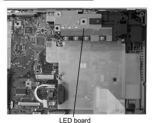
Lift up the **LED board** to disconnect it from PJ310 on the system board.
