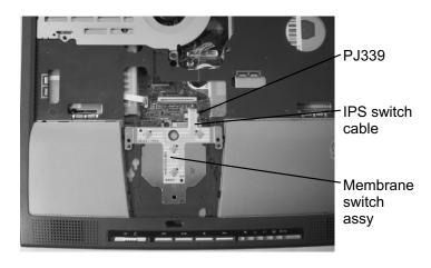
3. Disconnect the **IPS switch cable** from **PJ339** on the system board and lift out the **membrane switch assembly**.
