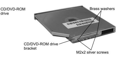
3. Remove two M2x2 silver screws and two brass washers securing the CD/DVD- ROM drive bracket.
