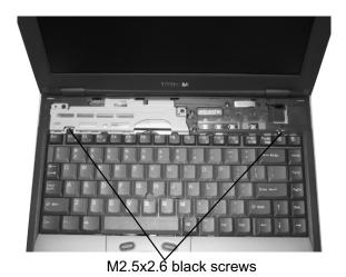
Remove two M2.5x2.6 black screws securing the keyboard.
