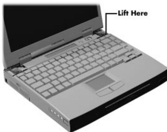
*Figure 2-15 Lifting the Keyboard*
