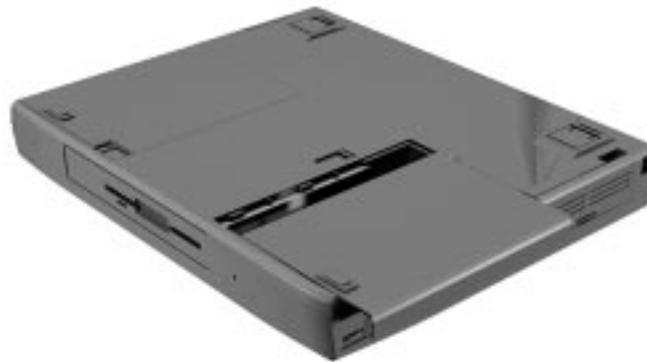
**Figure 2-8** *Replacing the Cover*
