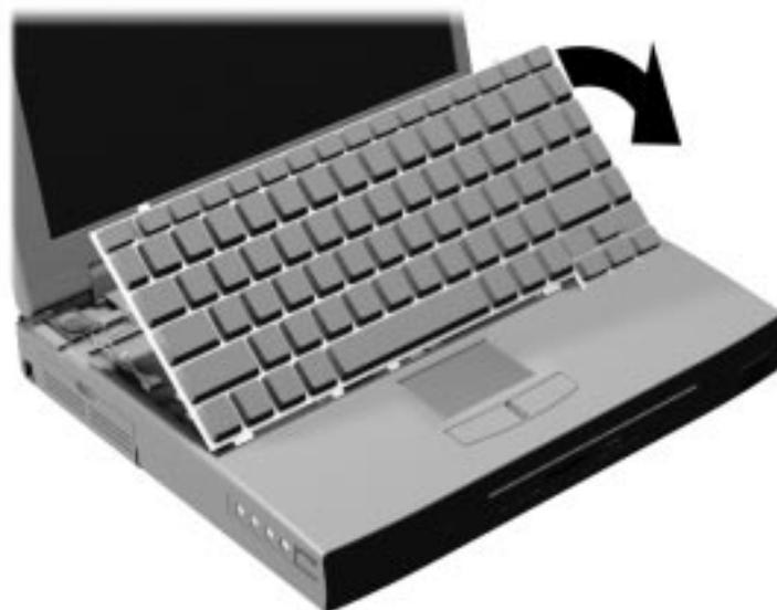
**Figure 4-10 Positioning the Keyboard**
