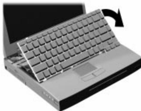
*Figure 2-16 Positioning the Keyboard*
