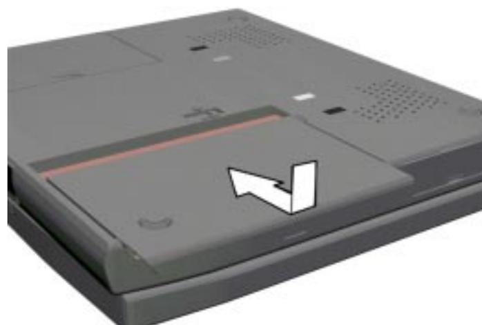
**Figure 2-8** *Replacing the Cover*
