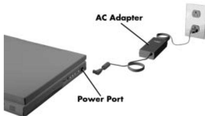
**Figure 2-1** Connecting the AC Adapter
