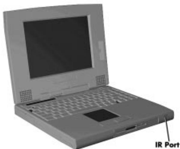
**Figure 1-8 Front IR Assembly Location**
