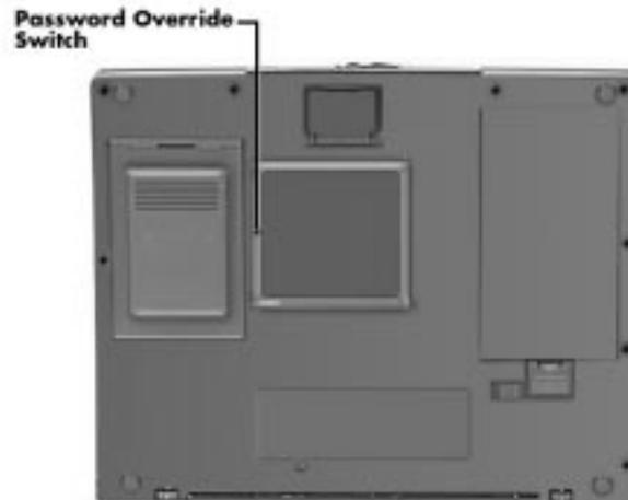
**Figure 2-11 Password Override Switch**
