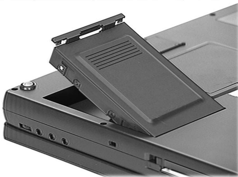
**Figure 4-8** *Removing the hard drive*
