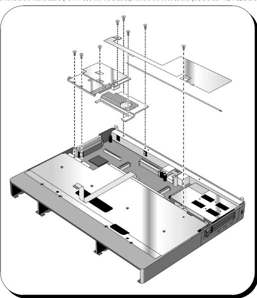
hold the PCA PT-586 in place. Remove the two standoffs (notice that one is 11.75mm long and the other is 15mm long). Remove the Dock Grounding Spring Plate. Remove the two PCMCIA buttons. Make sure that you have removed all RAM expansion modules. Then lift the PCA straight up. The I/O Bracket comes as part of the PCA PT-586. If only the I/O Bracket is damaged, it can be ordered separately and replaced by removing the 4 standoffs and two screws from the back of the bracket.
