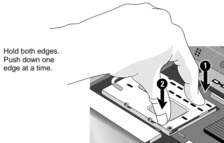
Figure 2-10. Inserting the CPU (OmniBook 4100/4150†)
