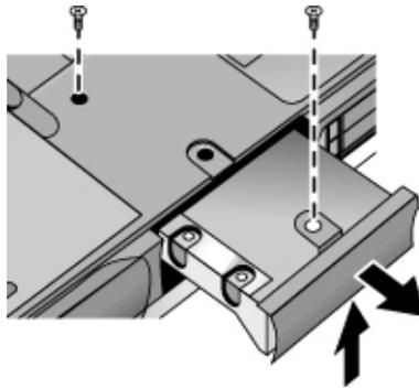
4. Gently slide the new drive into the hard drive compartment. Press firmly to make sure the connector seats properly.
