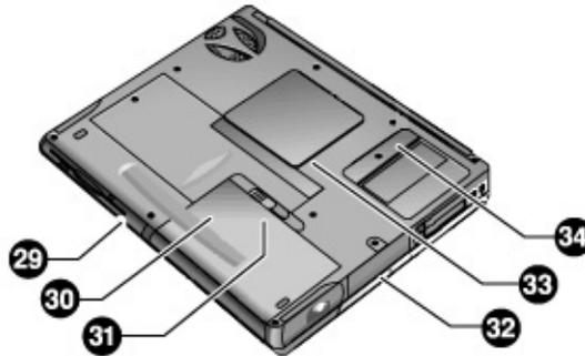
29. Plug-in module bay. Can contain a CD-ROM or DVD drive, floppy disk drive, secondary battery, or other plug-in module.
