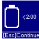
Low battery. Less than 2 minutes of battery life remain before automatic shut-down. Double beeps every 15 seconds remind you of this. Press ESC to acknowledge the message.
