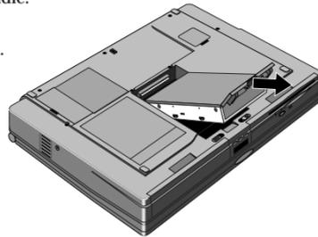
**Important:** After installing a new hard disk drive, you should create a Hibernate partition on the drive before loading any software—see the following instructions. Otherwise, the computer will not be able to enter Hibernate mode.
