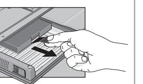
5 Pull out the hard disk using the black plastic tab, as shown.
