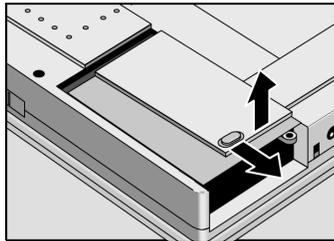
5. Release the two latches at the sides of the RAM board by pushing them outward and away from the sides of the module. When you release the latches, the free edge of the board pops up.
