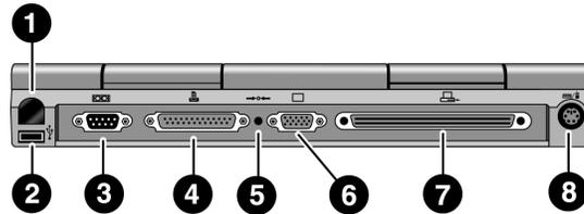
1. Infrared port. Use this port for wireless data transmission between the OmniBook and another computer or a printer with an infrared port. You must install infrared drivers. Windows NT 4.0 does not support infrared communication.
