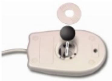
4. Remove any dust, lint, or dirt from the mouse ball with a soft cloth.
