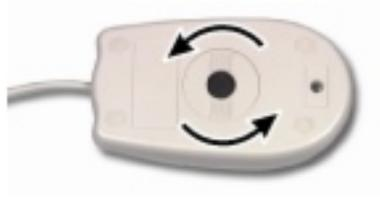
3. Remove the retaining ring and mouse ball.
