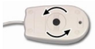
3. Remove the retaining ring and mouse ball.
