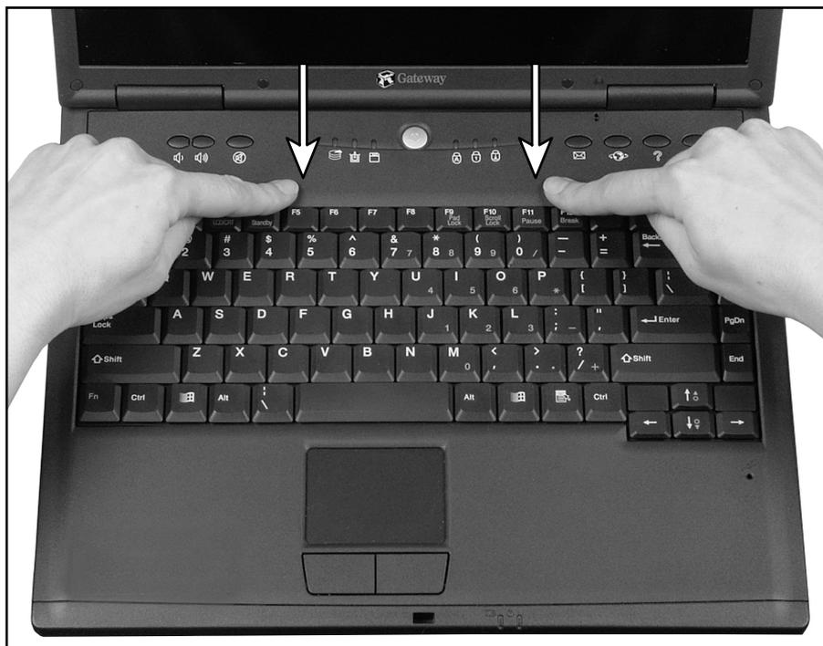
The bezel is correctly mounted when you can run your finger along the bezel and find no loose spots. The bezel should be flat all the way across. If the bezel is mounted incorrectly, complete the instructions under “Replacing the bezel” on page 12.
