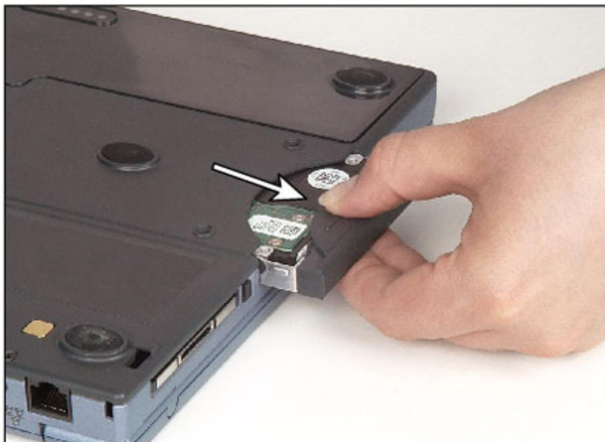
6. Insert the new hard drive kit in the bay until the outer edge of the kit is flush with the side of the notebook.
