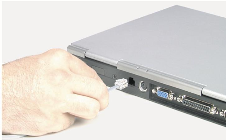
2. Insert the other end of the telephone cable into any analog telephone wall jack.
