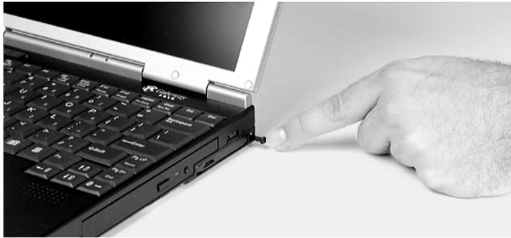
5. Press the PC Card eject button a second time to eject the PC Card.
