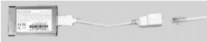
The combo PC Card modem (A) shown below has the 68-pin connector on one end and two ports (B, D) on the other end. The two ports include:
