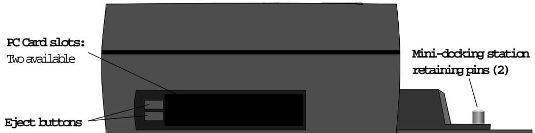
Figure 36. Mini-Docking Station - Right Side View
