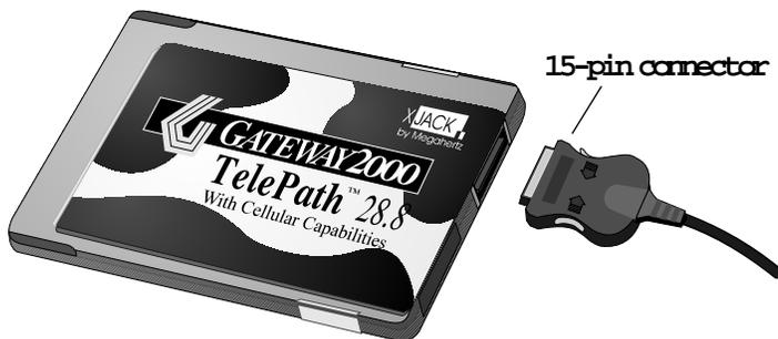
Figure 45. Making a 15-pin Connection
