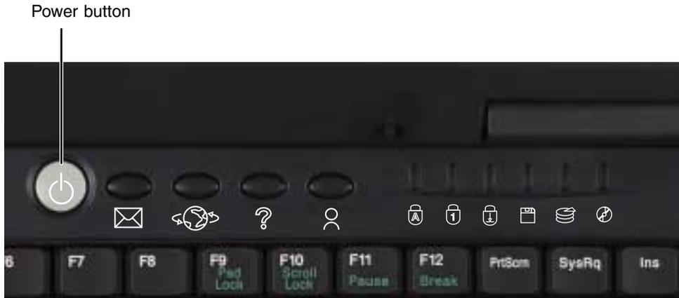
The power button is preset to On/Off mode. However, you can also set it to function in Standby/Resume mode. For instructions on changing the power button mode, see “Changing power settings” on page 137.
