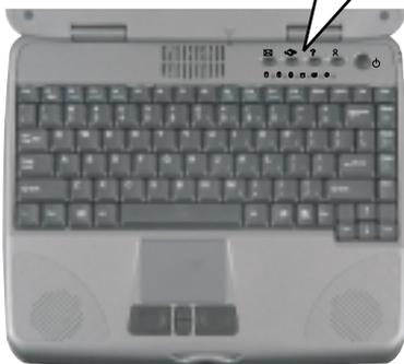
The power button is preset to On/Off mode. However, you can also set it to function in Standby/Resume mode. For instructions on changing the power button mode, see “Changing automatic power settings” on page 111.
