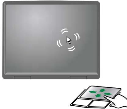
You can use the EZ-Pad *left* and *right* buttons below the touchpad to select objects. You can scroll using the rocker switch between the touchpad buttons. Scrolling capabilities are available in some Windows applications, including Microsoft Office.
