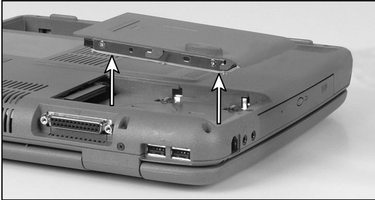
**7** Remove the four screws that attach the hard drive to the hard drive cover.
