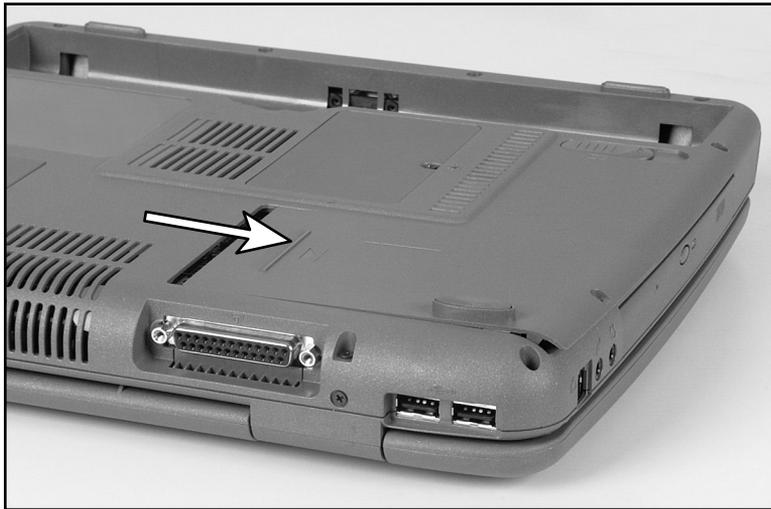
**6** Lift the hard drive kit out of the hard drive bay.
