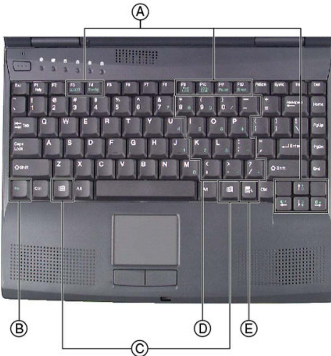
Your notebook features a full-size keyboard that has the full functionality of a desktop computer keyboard. Many of the keys have been assigned alternate functions, including shortcut keys for Windows, function keys for specific system operations, and Pad lock keys for the numeric keypad.
