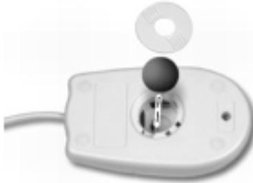
4. Remove any dust, lint, or dirt from the mouse ball with a soft cloth.
