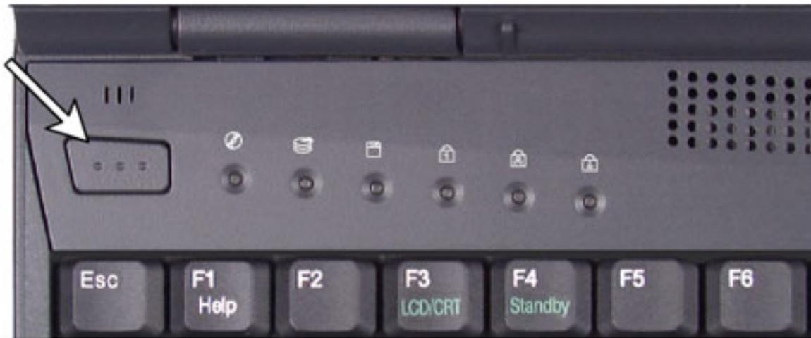
The power button is preset to On/Off mode. You can set it to function either in On/Off or Standby/Resume mode. See ["Changing power management settings"](#) for more information.
