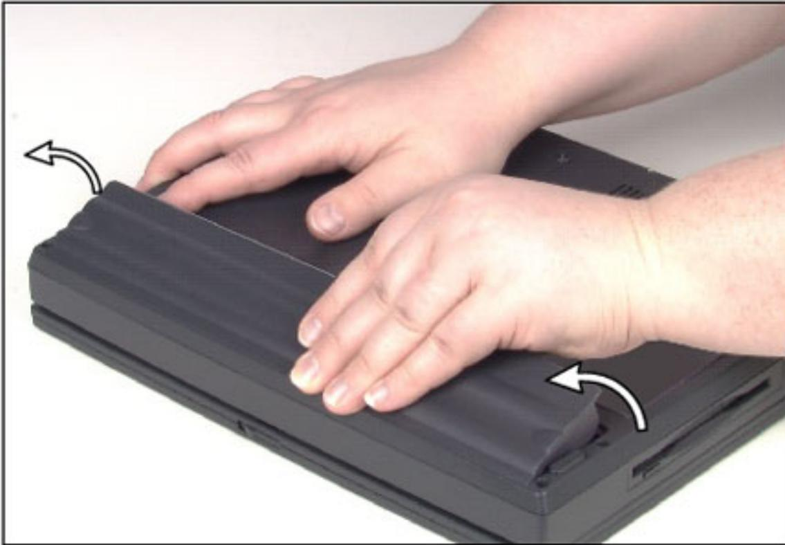
7. Slide the recharged battery into the bay and snap it into place.
