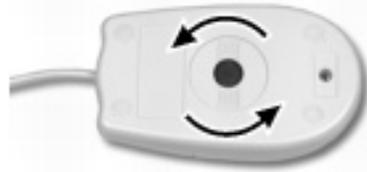
3. Remove the retaining ring and mouse ball.
