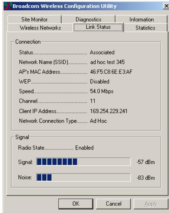
The top meter shows the signal strength for wireless Ethernet networking on your computer if access points or other computers with the same network name are within range of your computer.
