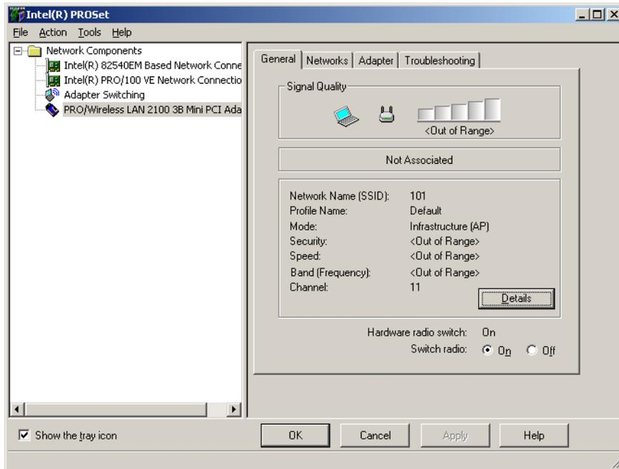
The meter at the top shows the signal strength for wireless Ethernet networking on your computer if access points or other computers with the same network name are within range of your computer. The status box in the middle provides status and error messages.
