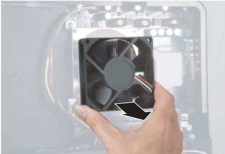
**7** Secure the new fan to the heatsink with the four screws removed in Step 4.
