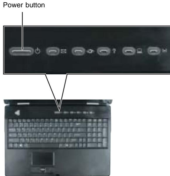
The power button is preset to On/Off mode. However, you can also set it to function in Standby/Resume mode. For instructions on changing the power button mode, see [“Changing power settings” on page 176](#).
