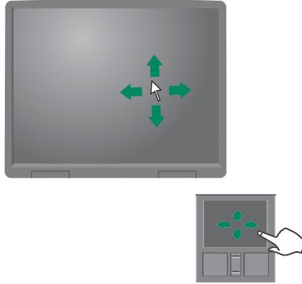
You can use the EZ-Pad *left* and *right buttons* below the touchpad to select objects. You can use the scroll wheel, located between the left and right buttons, to scroll your screen up and down.
