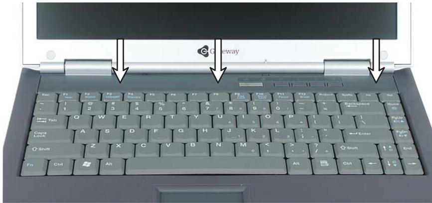
The bezel is correctly mounted when you can run your finger along the bezel and find no loose spots. The bezel should be flat all the way across.
