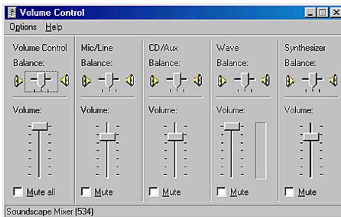
If the device you want to adjust does not appear in the *Volume Control* window, click **Options**, **Properties**, the audio device you want to adjust, then click **OK**.
