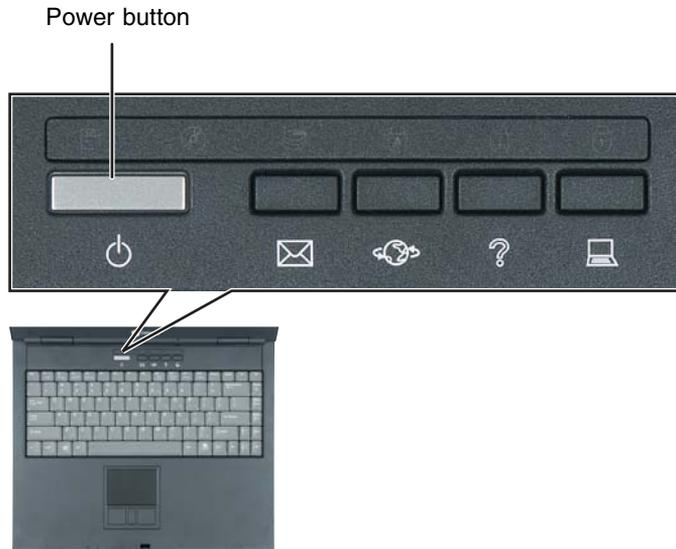
The power button is preset to On/Off mode. However, you can also set it to function in Standby/Resume mode. For instructions on changing the power button mode, see [“Changing power settings” on page 157](#).
