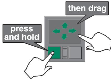
Position the pointer over the object. Press the left button and hold it down, then use the touchpad to move (drag) the object to the appropriate part of the screen. Release the button to drop the object where you want it.
