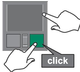
Position the pointer over the object. Quickly press and release the right button once. This action is called *right-clicking*.
