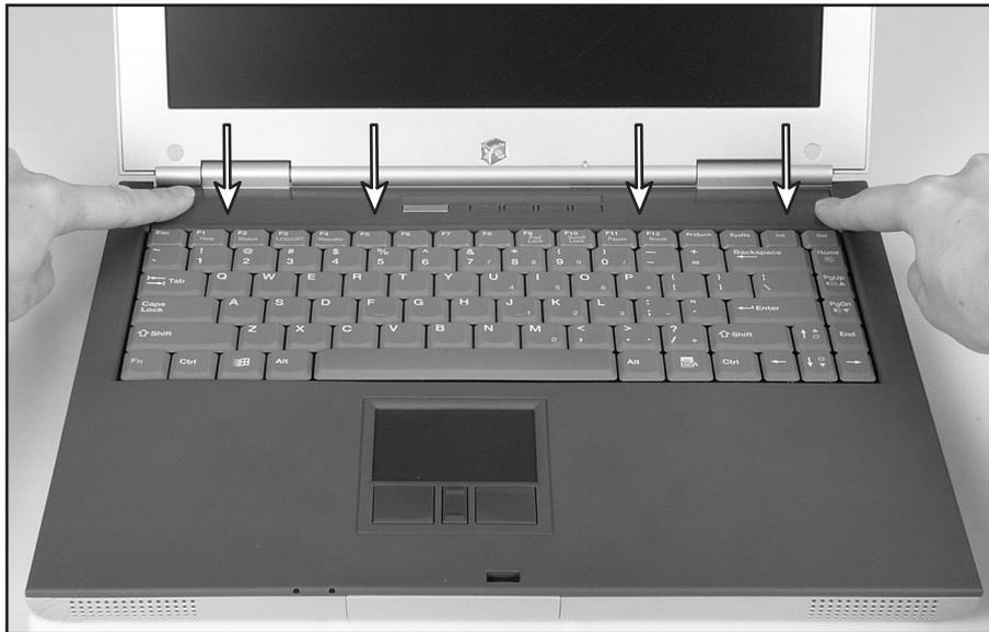
The bezel is correctly mounted when you can run your finger along the bezel and find no loose spots. The bezel should be flat all the way across. If the bezel is mounted incorrectly, complete the instructions under “Replacing the bezel” on page 12.
