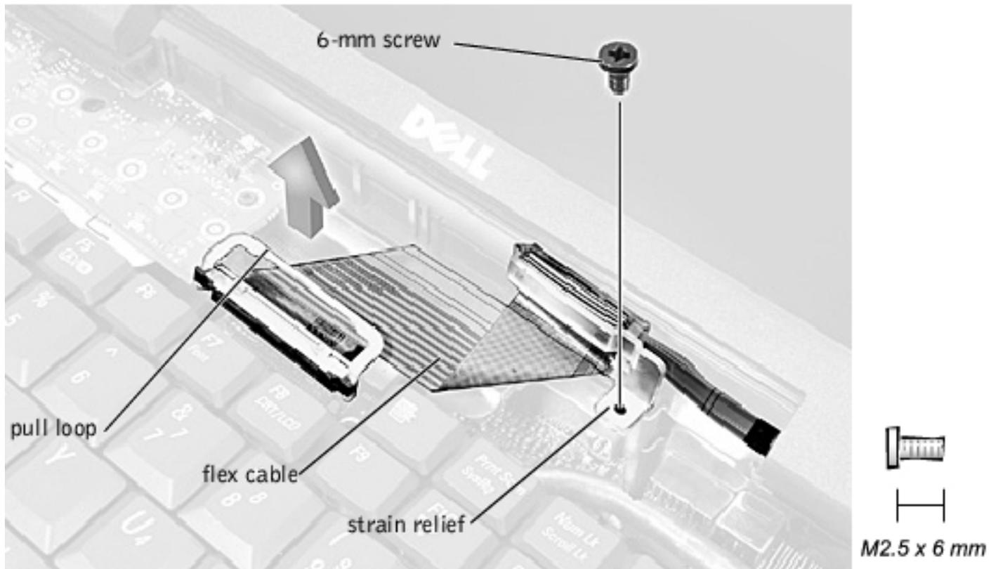
2. Remove the 6-mm screw that secures the display flex cable to the strain relief, and then use the pull loop to remove the display flex cable from the graphics card.
