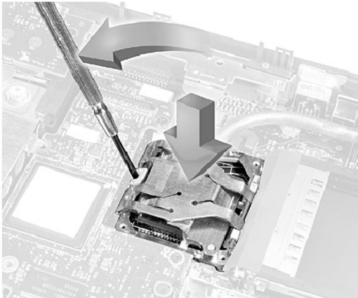
4. While pressing lightly down on the center of the retaining clip, insert a flat-blade
