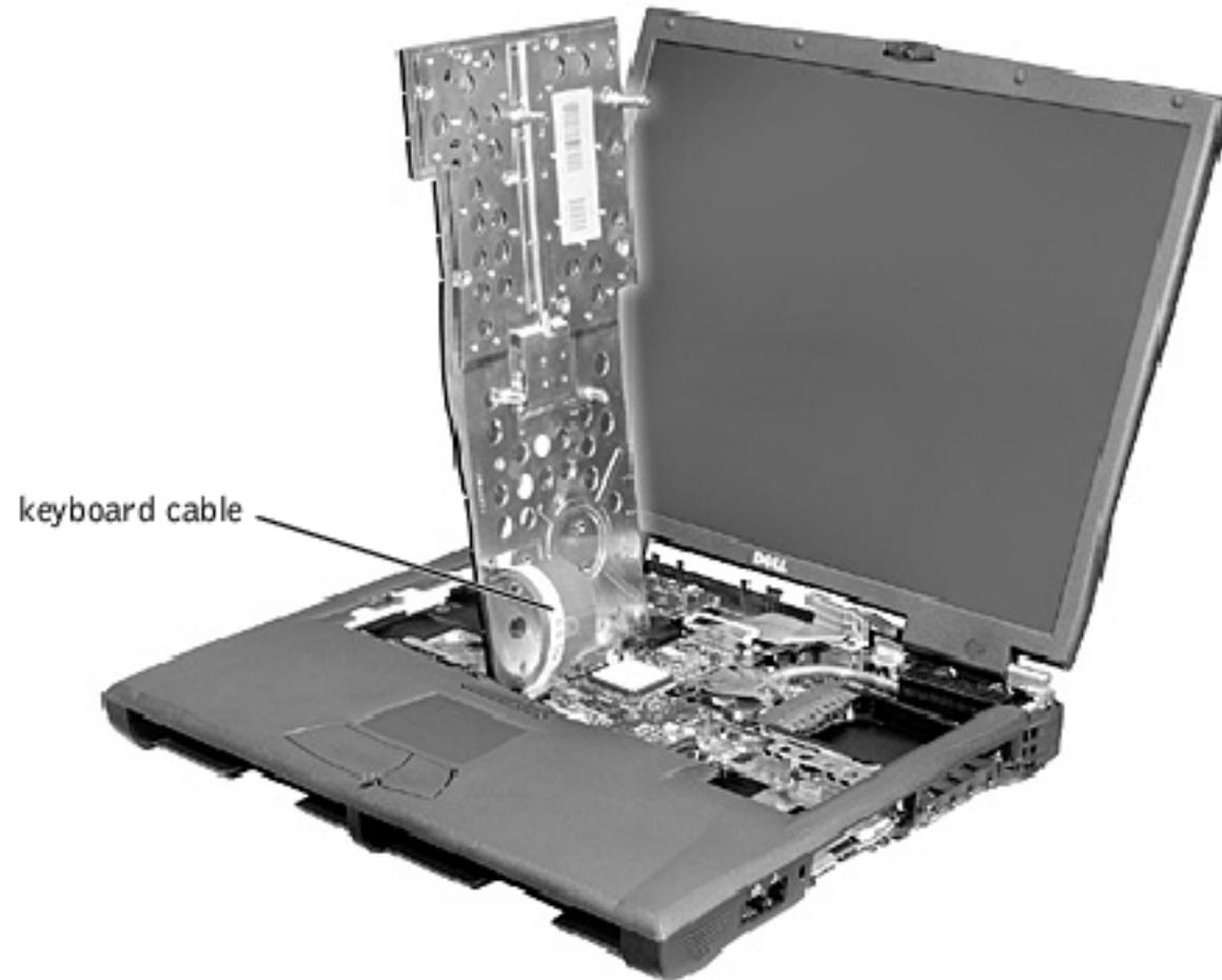
7. Disconnect the keyboard cable and lay the keyboard assembly aside.
