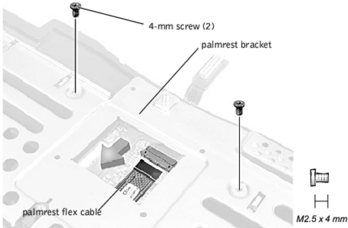
7. Remove the two 4-mm screws securing the palmrest bracket.
