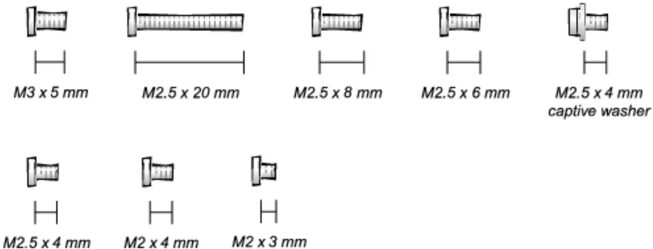
**➔ NOTICE:** When reinstalling a screw, you must use a screw of the correct diameter and length. Make sure that the screw is properly aligned with its corresponding hole, and avoid overtightening.
