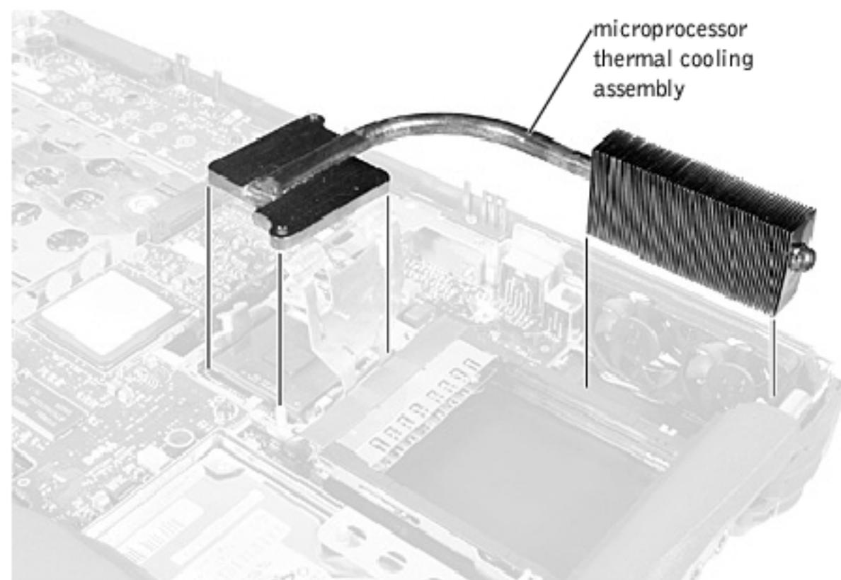
**NOTICE:** To ensure maximum cooling for the microprocessor, do not touch the heat transfer areas on the microprocessor thermal cooling assembly. The oils in your skin reduce the heat transfer capability of the thermal pads.
