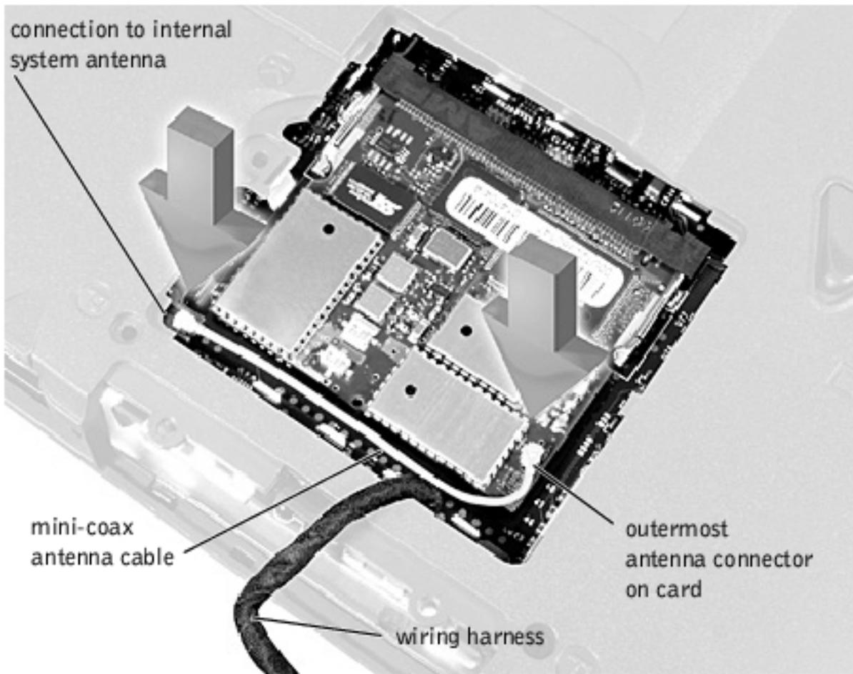
➔ **NOTICE:** If a wireless NIC card contains two mini-coax antenna connectors, connect the mini-coax antenna cable to the outermost antenna connector on the card as shown.
