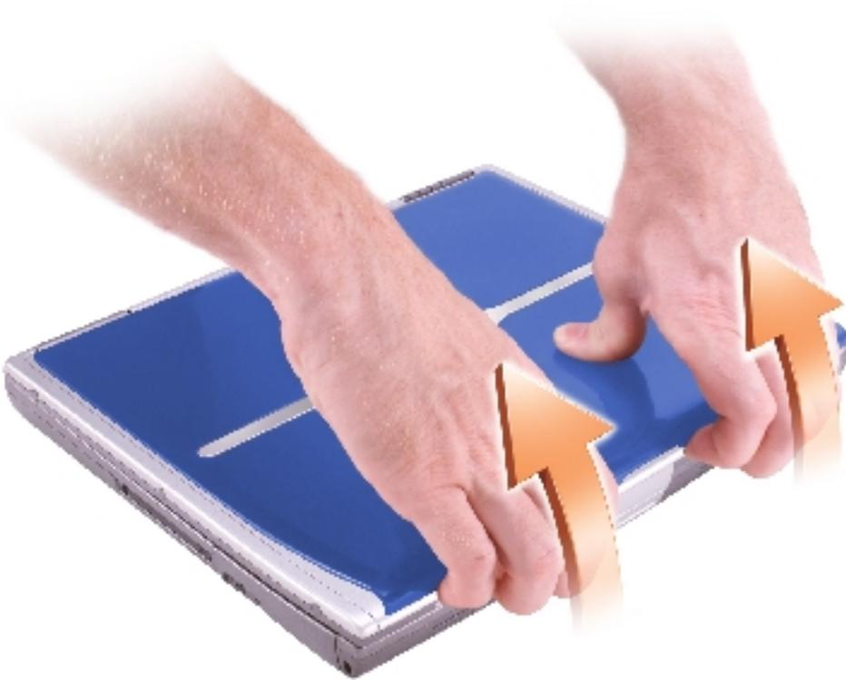
2. Firmly grasp the lip of the cover to detach it from the computer, and pull the cover up.
