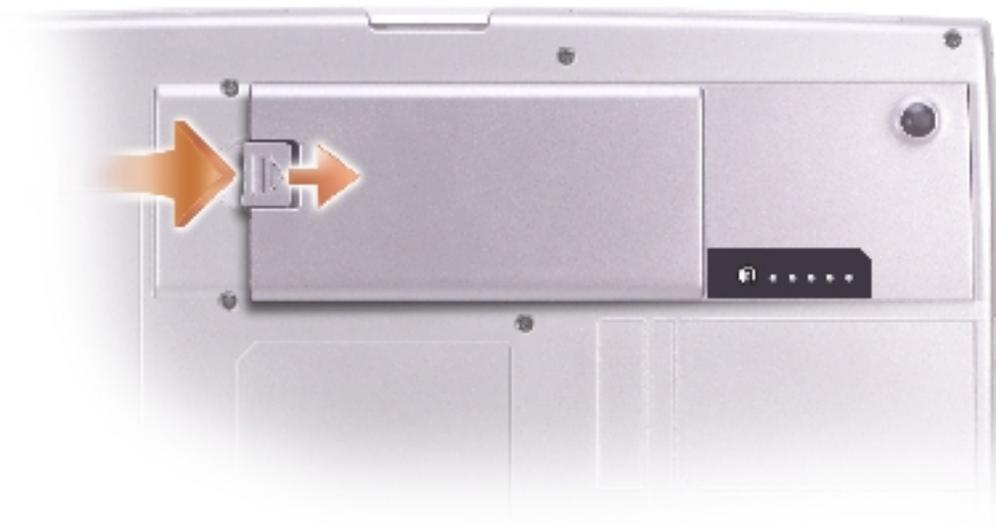
11. Remove any installed [memory modules](#), [Mini PCI cards](#), and [modules](#), including a second battery if one is installed.
