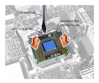
Use the microprocessor extraction tool to remove the microprocessor module.
