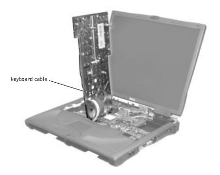
7 Disconnect the keyboard cable and lay the keyboard assembly aside.
