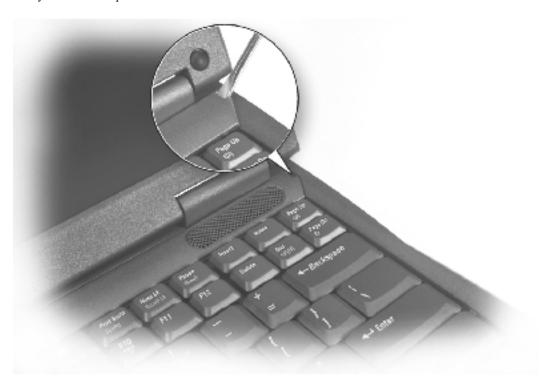
5. To release the keyboard from the palm rest, use a small, flat-blade screwdriver or plastic scribe to pull up on the right edge of the blank key on the keyboard.
