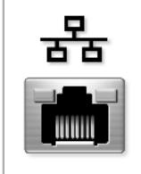
Connects the computer to a network. The lights next to the connector indicate activity for both wired and wireless network communications.
