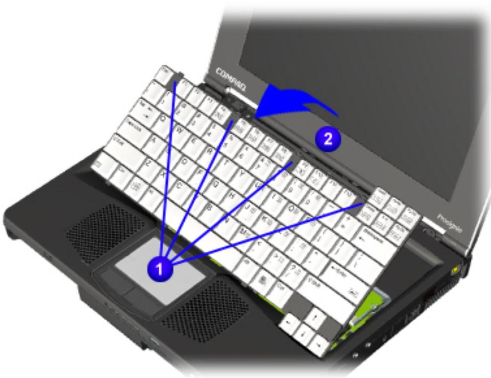
4 Slide the four tabs located along the top of the keyboard **1** towards the front of the computer.
