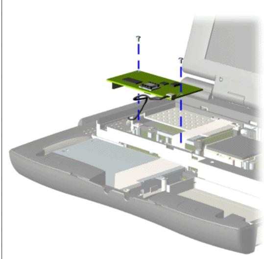
To remove the modem, complete the following steps:
