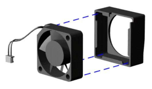
To remove the fan gasket, complete the following step:
