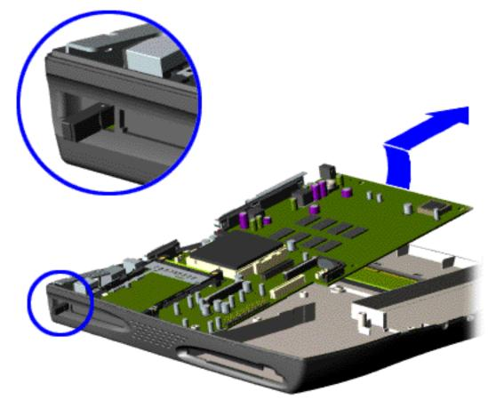
18. Pull the PCMCIA eject lever out (straight), lift up the right side of the system board and pull forward to remove the system board from the chassis.
