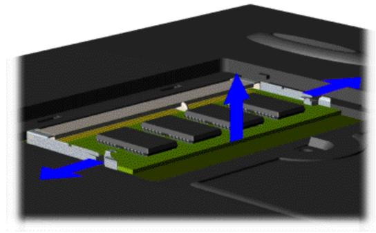
4. Pull side levers to release the memory module and unplug the memory module from the system board.
