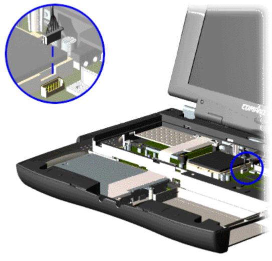
8. Disconnect the backlight cable attached to the display panel assembly from the connector on the system board.
