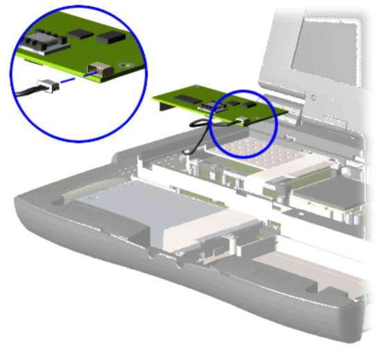
6. Disconnect the modem cable from the modem.
