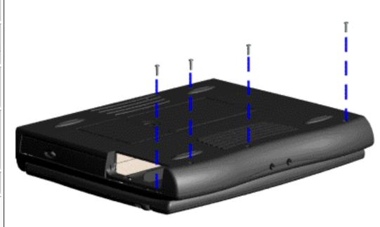
The palmrest cover with touch pad must be removed to gain access to any of the interior components of the computer, and it is the first component that has to be removed to gain access to the interior components.
