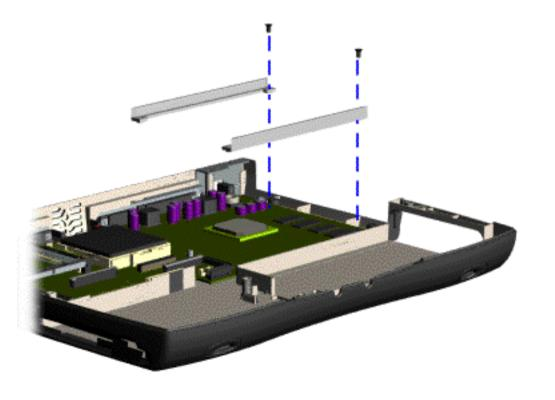
16. Remove two screws from the CD Drive mounting rails and remove the mounting rails from the system board.
