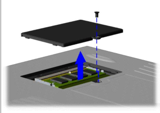
To remove the memory module, complete the following steps:
