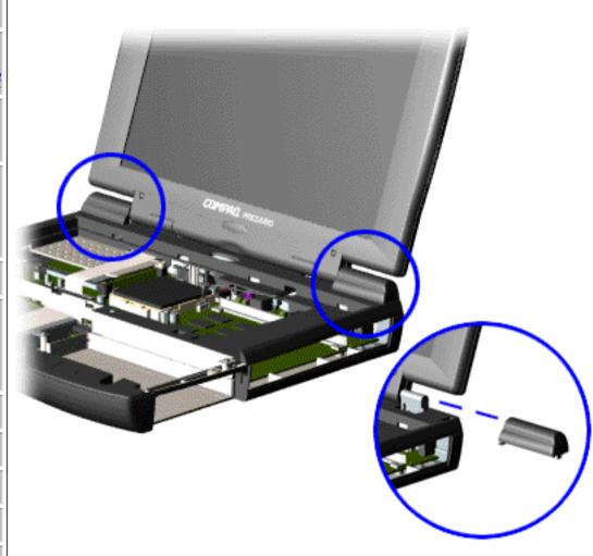
To remove the display panel assembly, complete the following steps:
