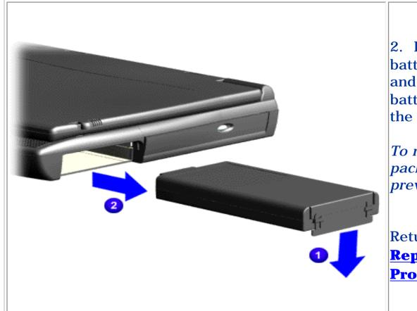
2. Pull forward on the battery pack tab <sup>1</sup> and remove the battery pack <sup>2</sup> from the chassis.
