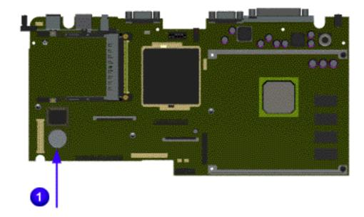
Clearing the power-on password requires removing all Setup attributes that are programmed in the CMOS. The RTC battery 1 is located on the system board.
