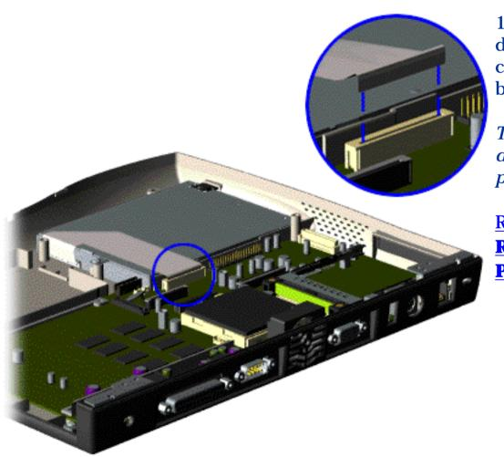
10. Disconnect the diskette drive data cable from the system board.
