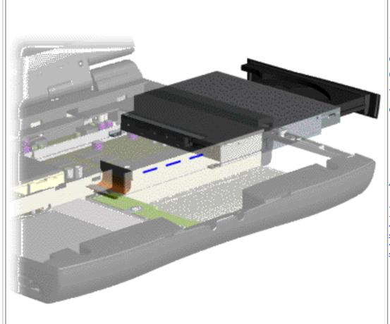
7. Disconnect the CD drive cable from the CD drive and remove the CD drive from the chassis.
