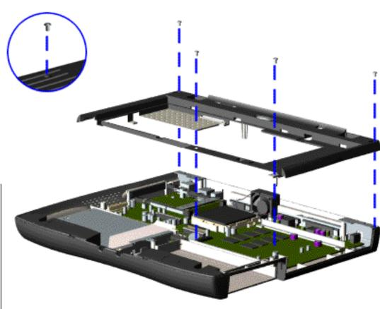
To remove the Upper CPU cover complete the following steps:
