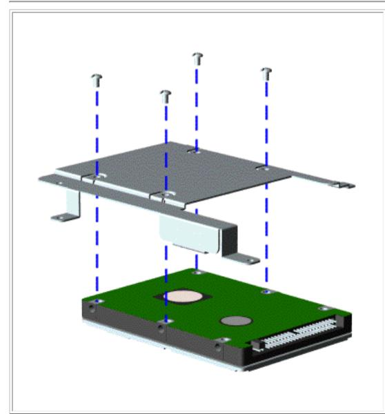
To remove the hard drive mounting bracket, remove four screws from the mounting bracket as shown in the illustration.
