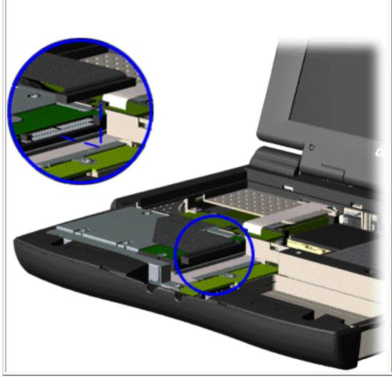
5. Disconnect the hard drive data cable from the hard drive and remove from the chassis.
