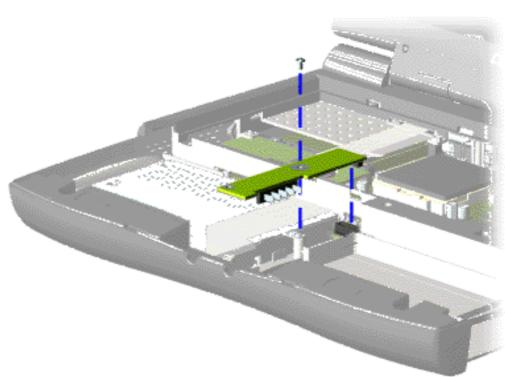
To remove the battery charger board, complete the following steps:
