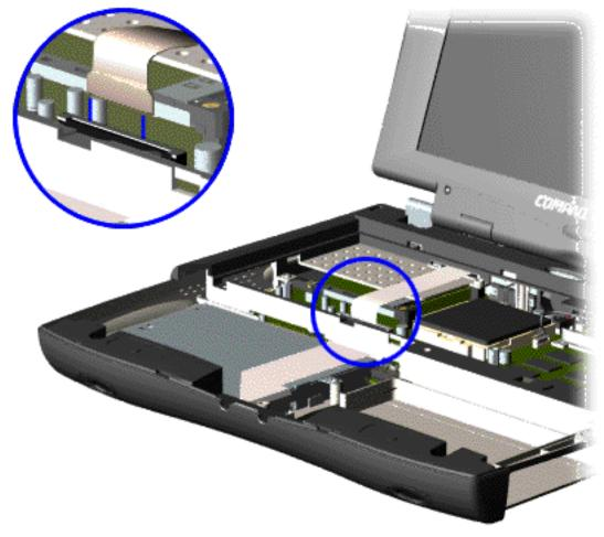
7. Disconnect the flex cable attached to the display panel assembly from the ZIF connector on the system board.
