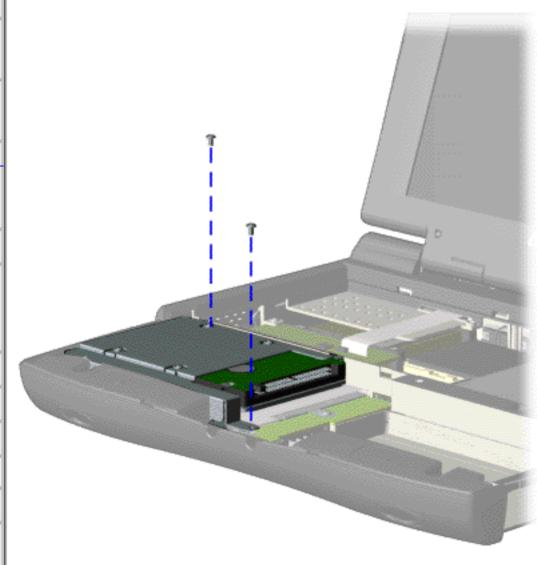
To remove the hard drive, complete the following steps:
