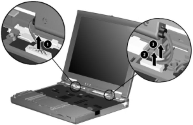
**Figure 5-25.** *Disconnecting the Display Cables*
