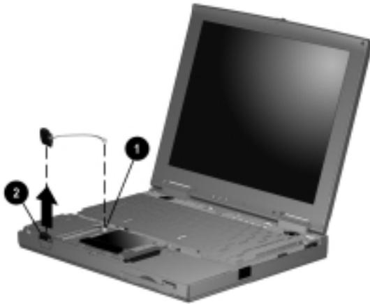
**Figure 5-18.** Removing the RTC Battery
