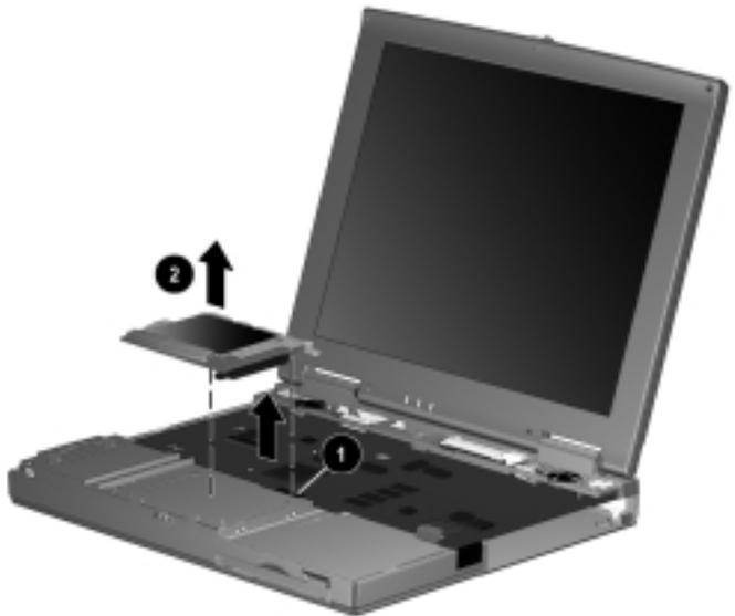
**Figure 5-22.** Removing the TouchPad
