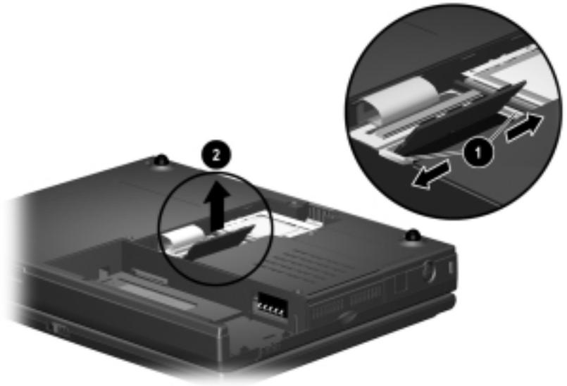
**Figure 5-13.** Removing a Memory Expansion Board
