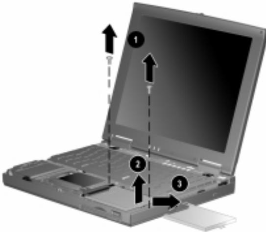
**Figure 5-17.** Removing the Hard Drive
