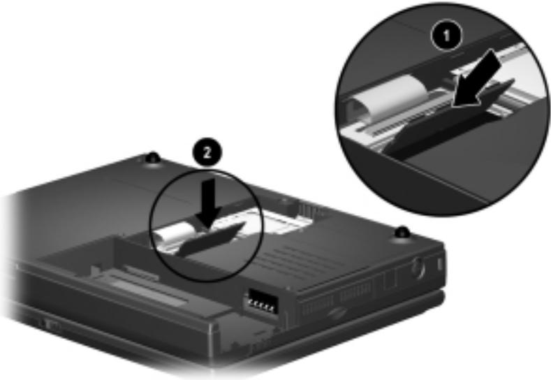
**Figure 5-14.** *Installing a Memory Expansion Board*
