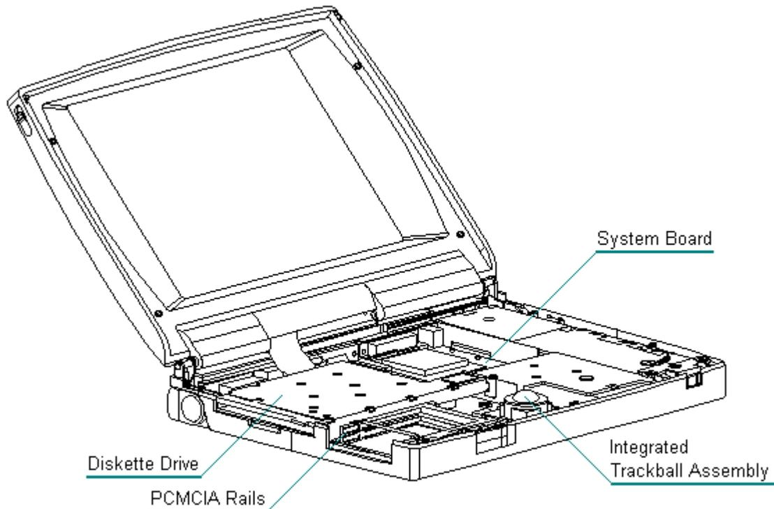
Figure 1-3. System Unit Module for Models 400 and 410
