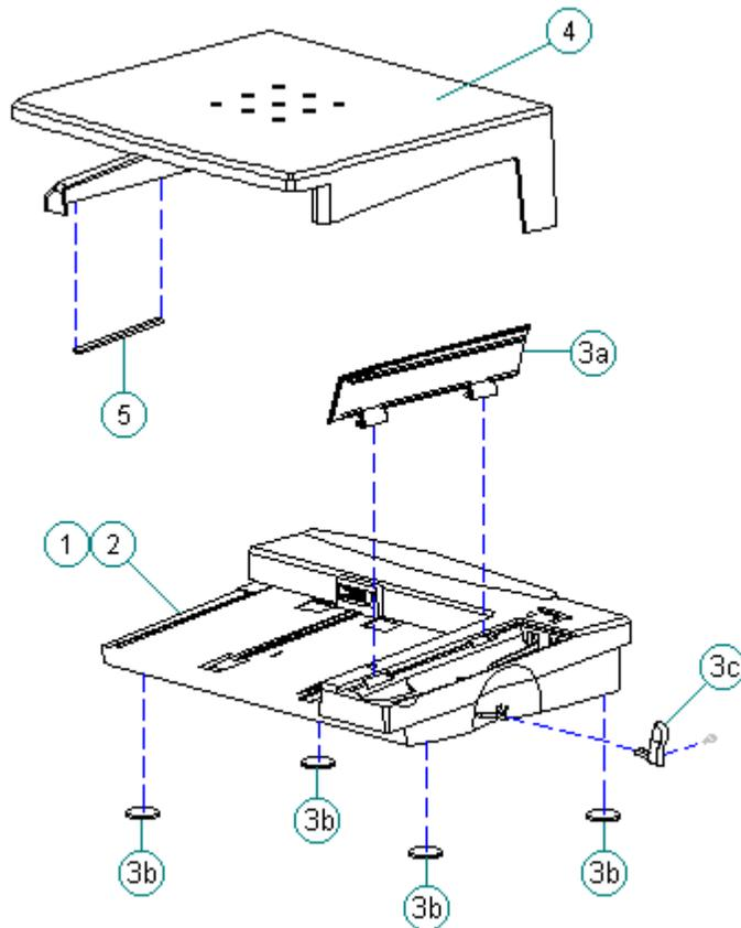
Figure 1-23. Docking Base and Monitor Support Cover (All Models)
