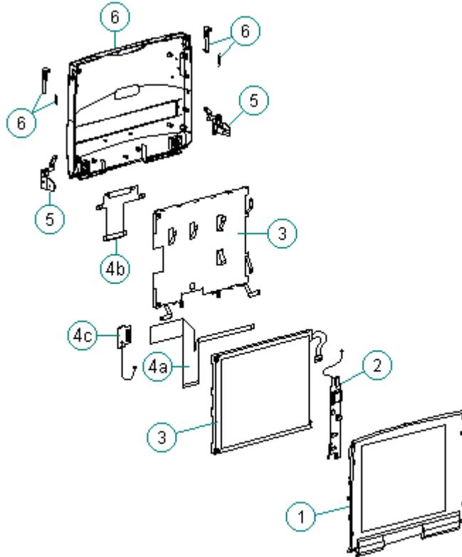
Figure 1-13. CSTN (10.4 inch) Display Assembly for Models 420 and 430
