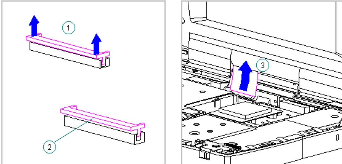
Figure 3-101. Removing the Display Cable from the System Board (Models 400 and 410)
