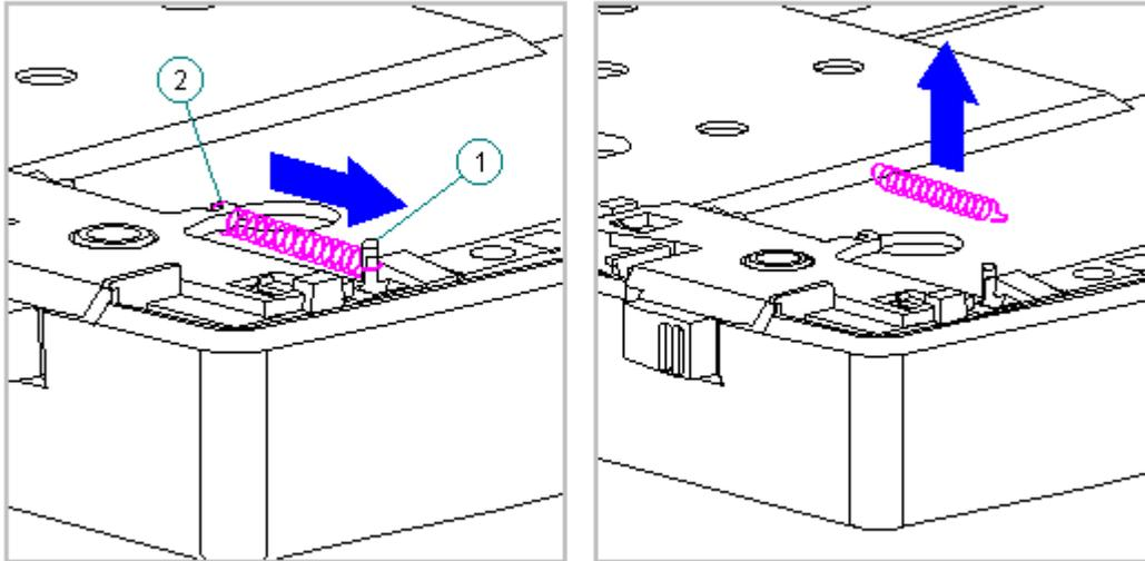
Figure 3-32. Removing the Battery Release Button Spring (All Models)
