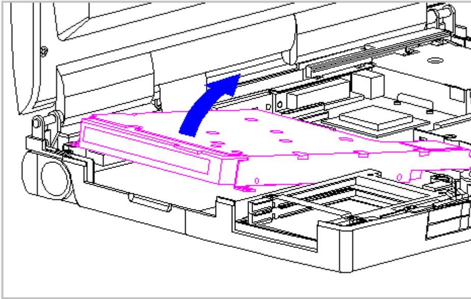
Figure 3-43. Removing the Diskette Drive from the System Chassis (All Models)
