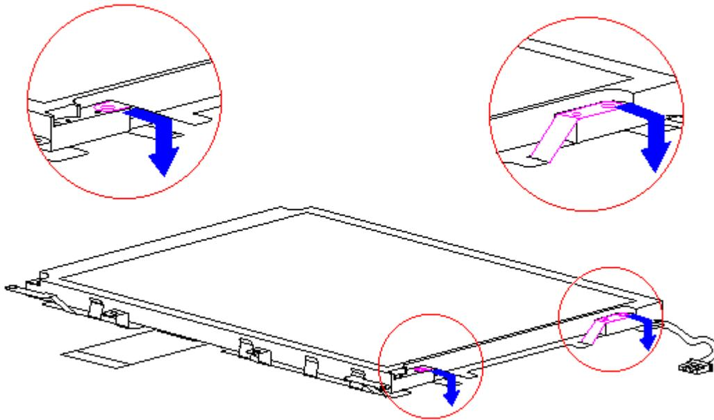
Figure 3-145. Removing the Display Shield Tabs (Models 420 and 430)
