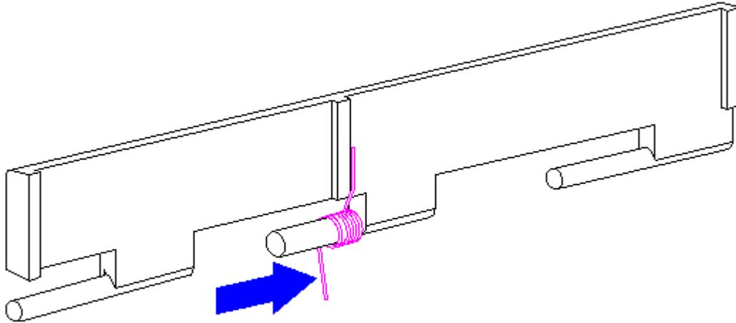
Figure 3-66. Replacing the PC Card Spring (All Models)
