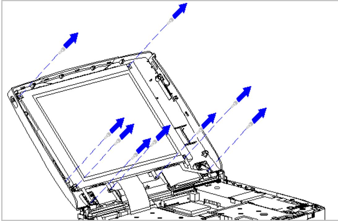
Figure 3-89. Removing the Screws from the Monochrome LCD Panel and the Shield (Models 400 and 410)
