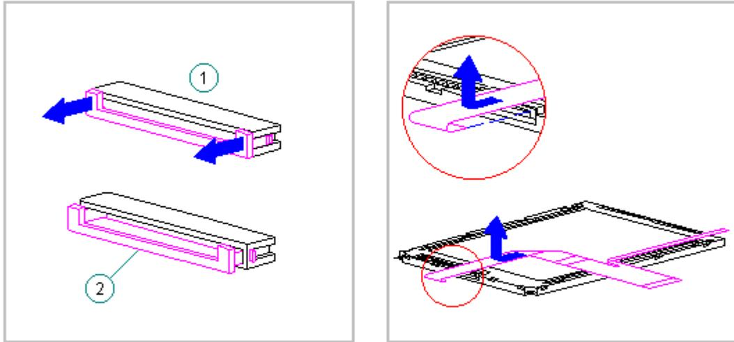
Figure 3-92. Removing the Display Cable from the Monochrome LCD Panel (Models 400 and 410)
