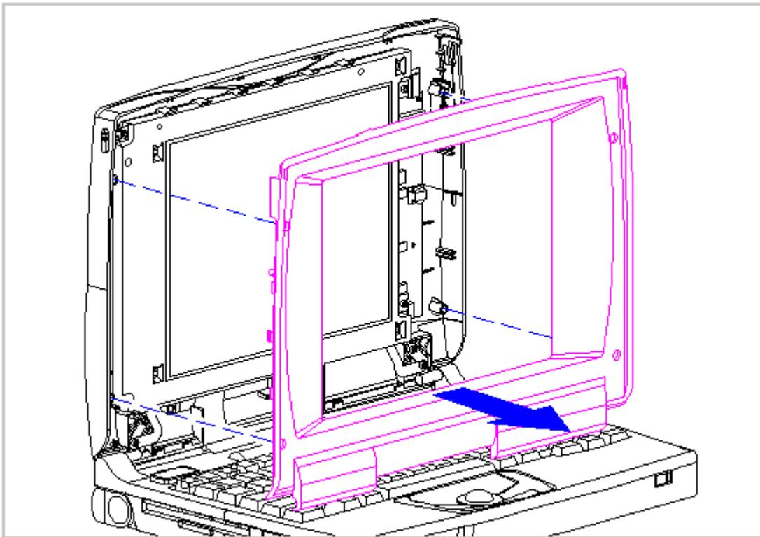
Figure 3-79. Removing the Display Bezel (Models 400 and 410)
