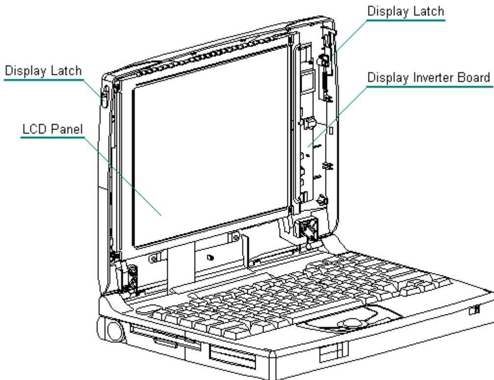
Figure 1-5. Display Assembly for Models 400 and 410
