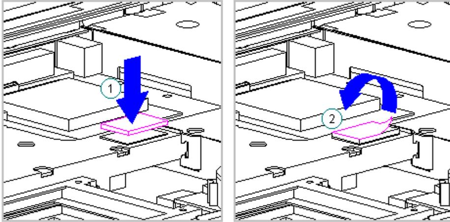
Figure 3-27. Attaching the Hook and Loop Fastener (All Models)
