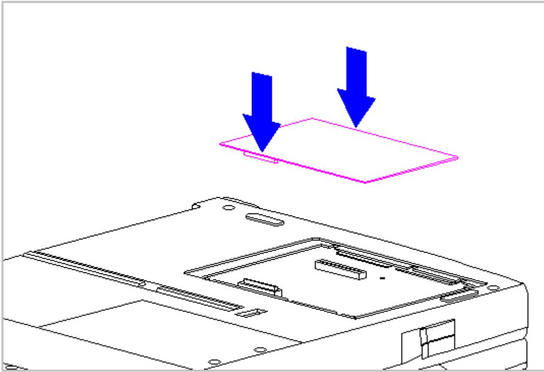
Figure 3-16. Replacing the Memory Expansion Board (All Models)
