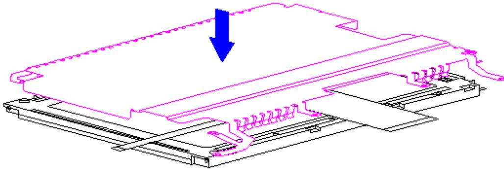
Figure 3-96. Placing the Shield on the Monochrome LCD Panel (Models 400 and 410)
