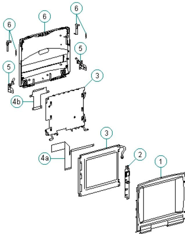
Figure 1-12. CSTN (9.5 inch) Display Assembly for Models 400 and 410
