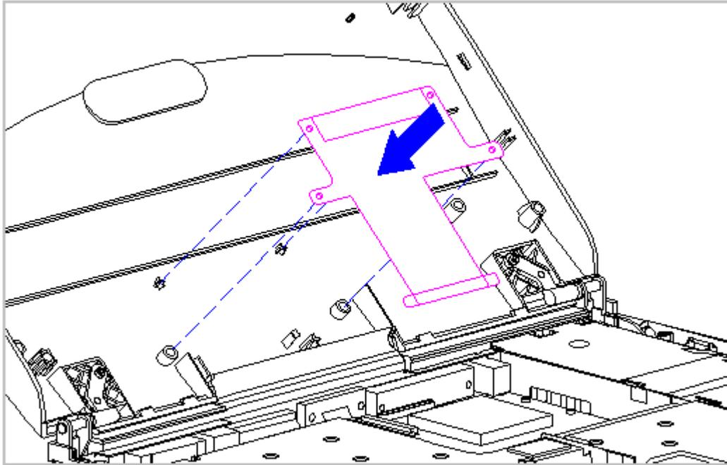
Figure 3-150. Replacing the Display Ground Cable (Models 420 and 430)
