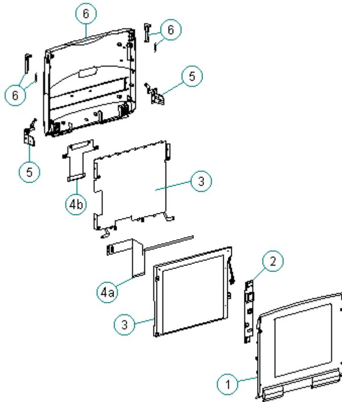
Figure 1-15. CTFT (10.4 inch) Display Assembly for Models 420 and 430
