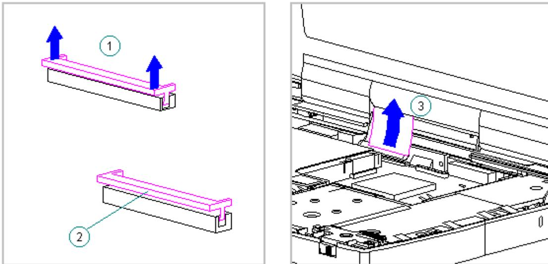
Figure 3-171. Disconnecting the Display Cable from the System Board (All Models)
