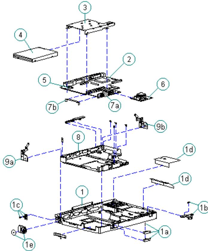
Figure 1-10. System Unit Module Parts for Models 420 and 430
