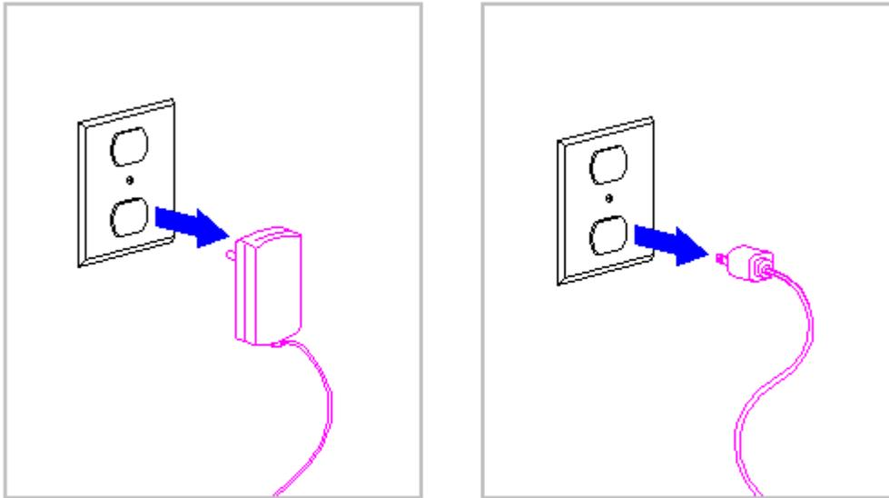
Figure 3-1. Disconnecting the AC Adapter from the Electrical Outlet
