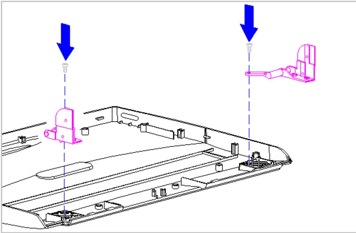
Figure 3-176. Replacing the Display Clutches (All Models)
