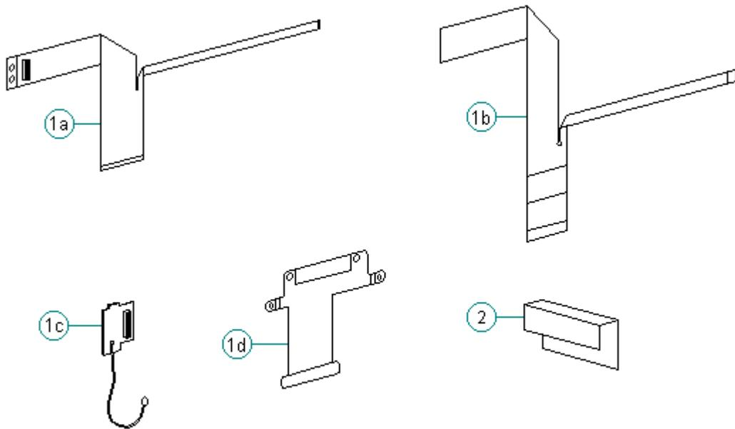
Figure 1-19. Cables for Models 420 and 430
