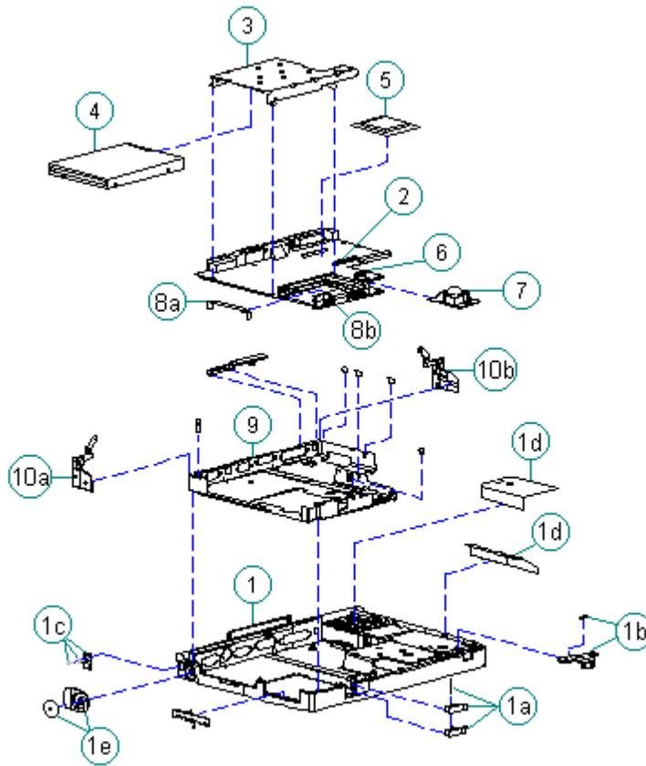
Figure 1-9. System Unit Module Parts for Models 400 and 410
