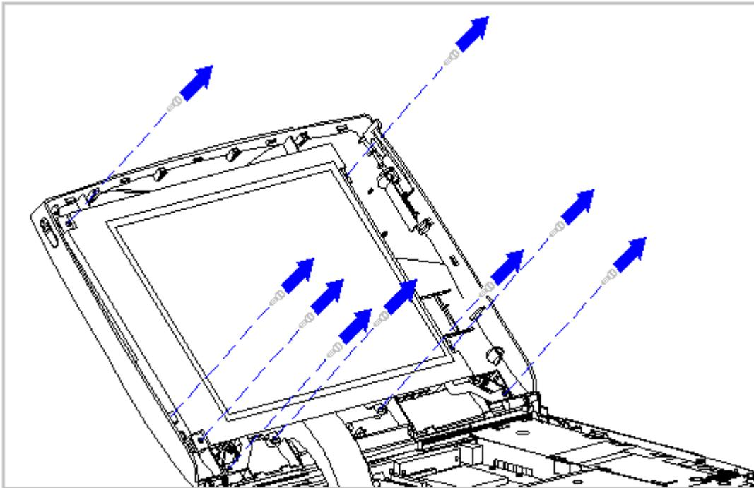
Figure 3-104. Removing the Screws from the CSTN (9.5 inch) Panel and Shield
