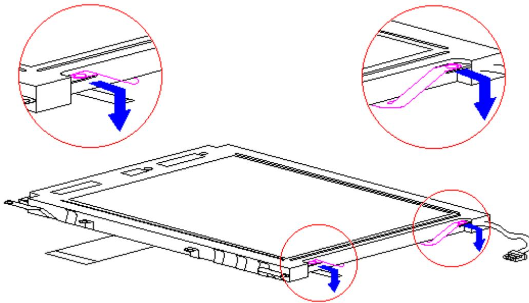
Figure 3-106. Removing the Display Shield Tabs (Models 400 and 410)
