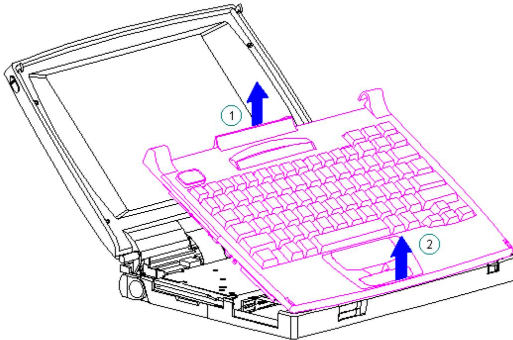
Figure 3-21. Removing the Keyboard Assembly (All Models)
