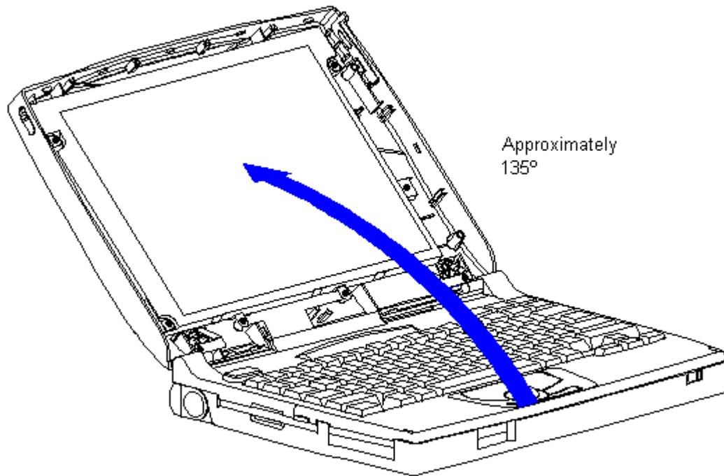
Figure 3-158. Opening the Display to Approximately 135-Degree Angle
