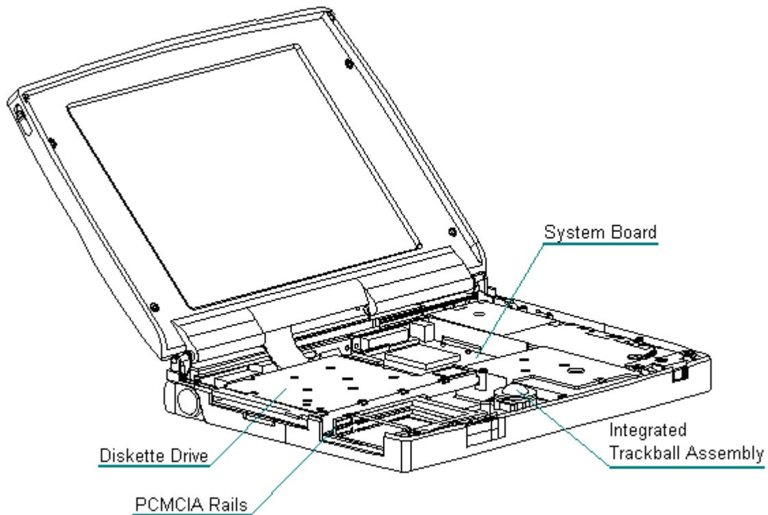
Figure 1-4. System Unit Module for Models 420 and 430
