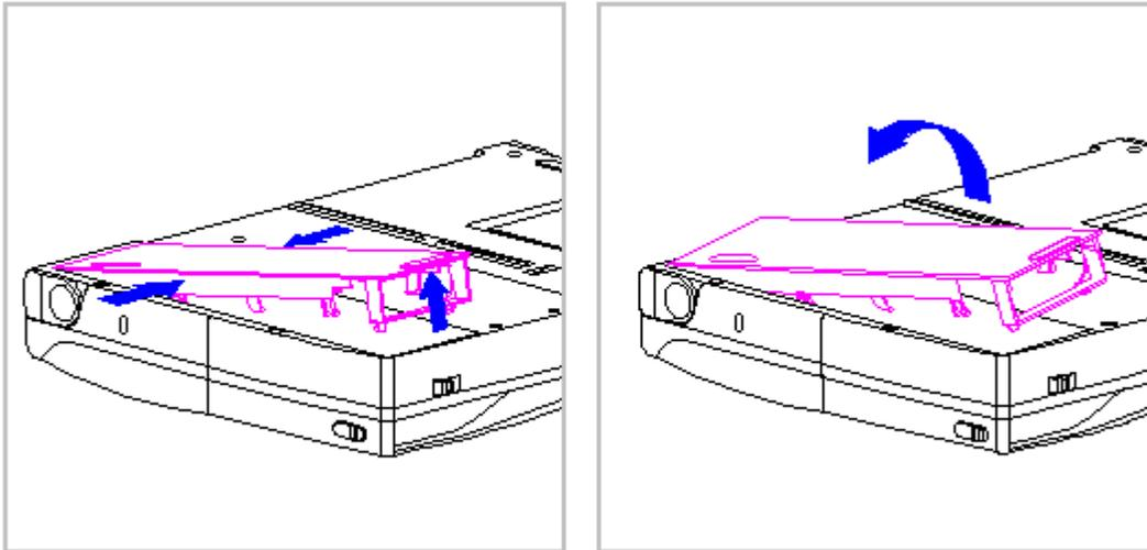
Figure 3-30. Removing the Battery Compartment (All Models)
