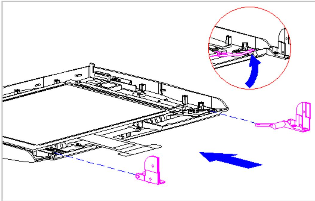
Figure 3-191. Replacing the Display Clutches (All Models)
