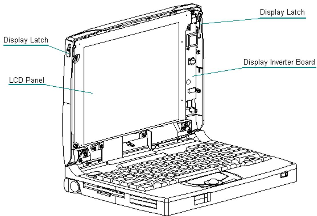
Figure 1-6. Display Assembly for Models 420 and 430
