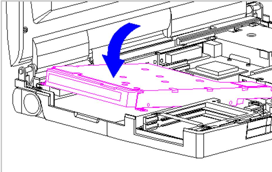
Figure 3-47. Replacing the Diskette Drive (All Models)
