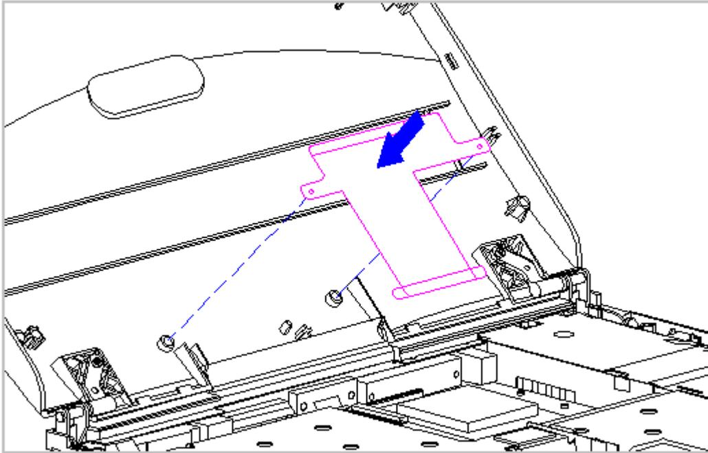
Figure 3-94. Replacing the Display Ground Cable (Models 400 and 410)
