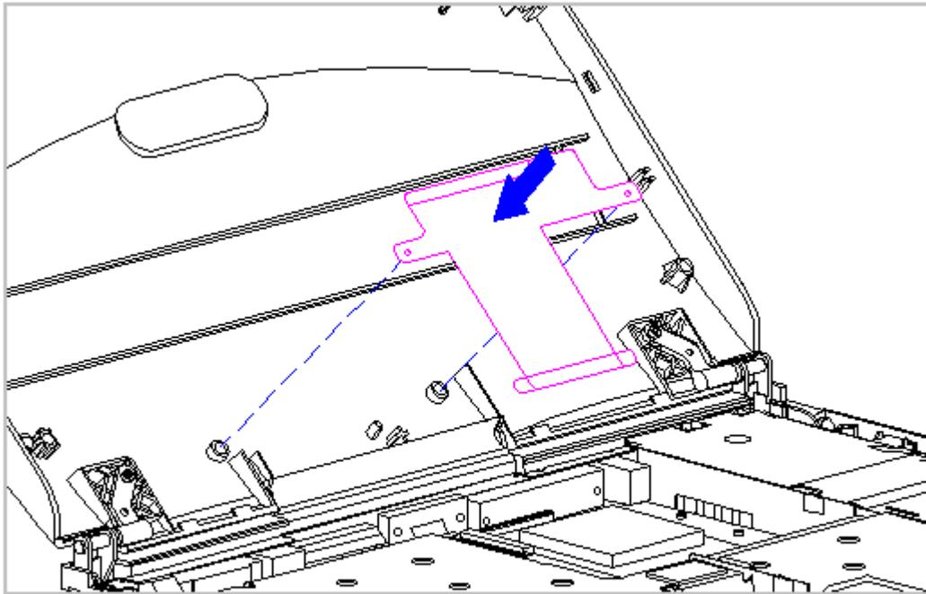
Figure 3-110. Replacing the Display Ground Cable (Models 400 and 410)
