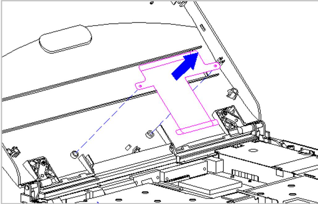
Figure 3-128. Removing the Display Ground Cable (Models 400 and 410)
