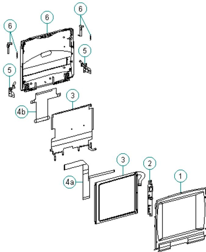
Figure 1-11. Monochrome Display Assembly for Models 400 and 410
