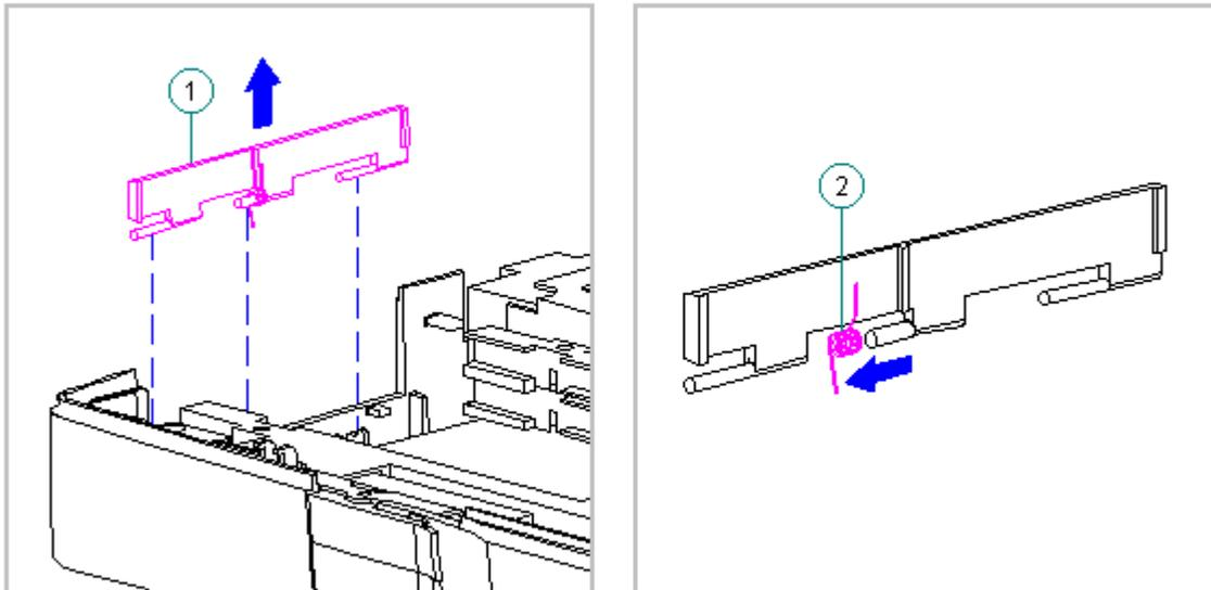
Figure 3-68. Removing the Bottom PC Card Door and Spring (All Models)
