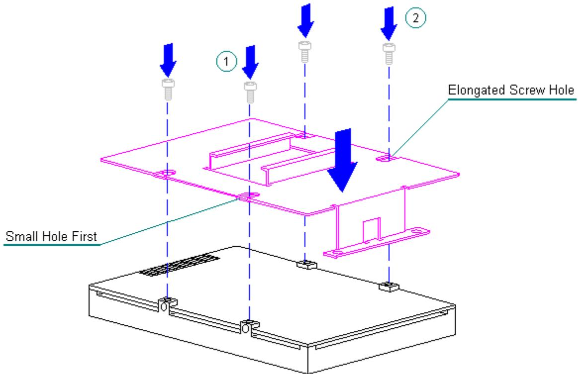
Figure 3-12. Replacing the Hard Drive Bracket (All Models)
