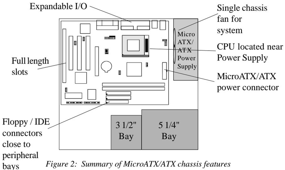
Figure 2: Summary of MicroATX/ATX chassis features
