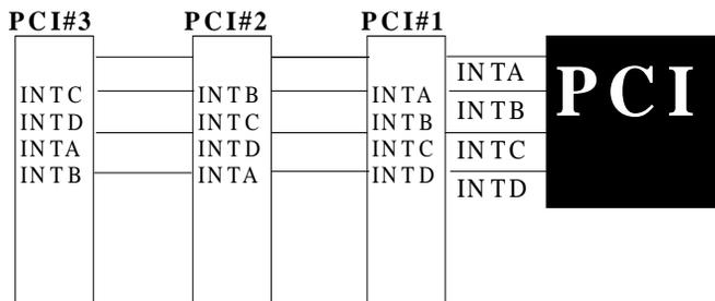
**Figure 7: The Combination of PCI INT#lines**
