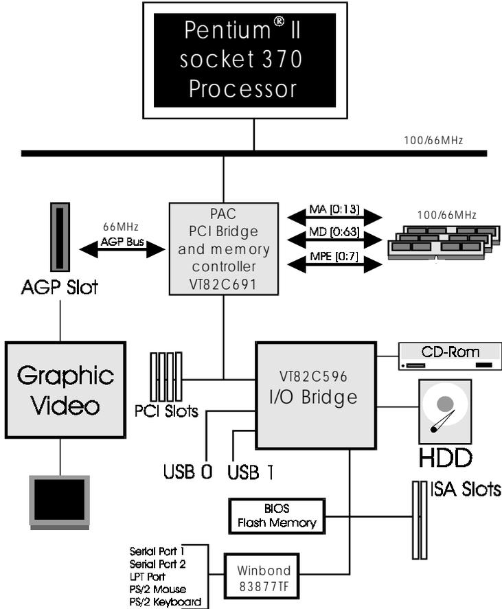
Figure 5: System Block Diagram
