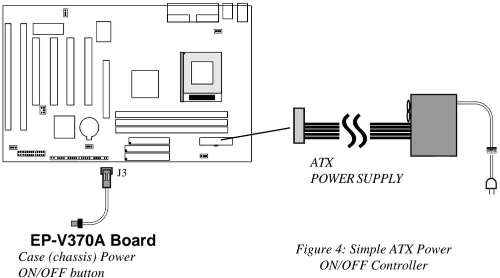
Figure 4: Simple ATX Power ON/OFF Controller
