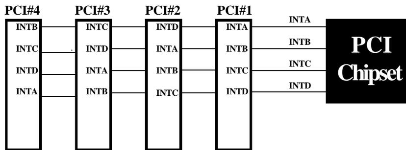
**Figure 3-7 The Combination of PCI INT# lines**
