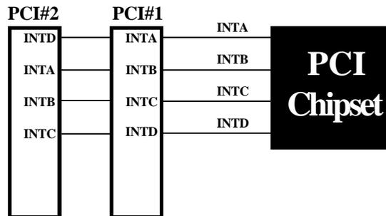
**Figure 3-7 The Combination of PCI INT# lines**
