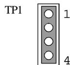
1-2, 3-4 CLOSE To Disabled Onboard U28,U29 SRAM Chips
