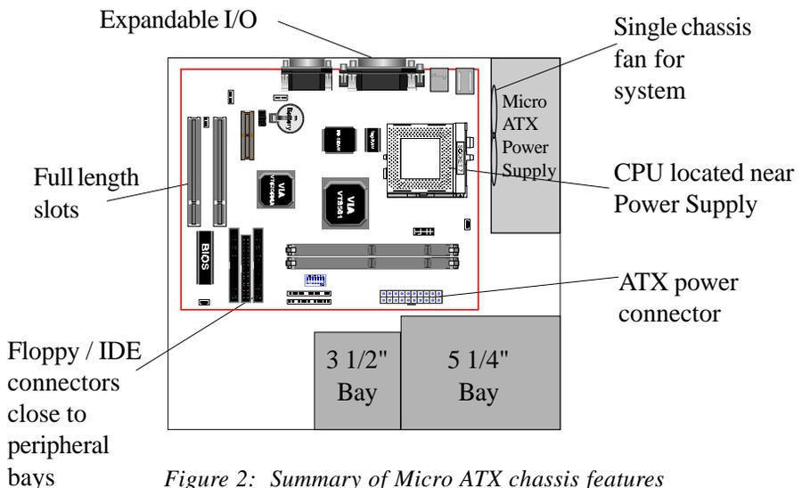
Figure 2: Summary of Micro ATX chassis features
