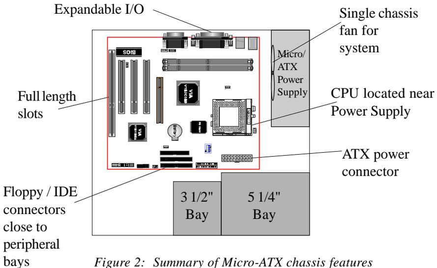
Figure 2: Summary of Micro-ATX chassis features
