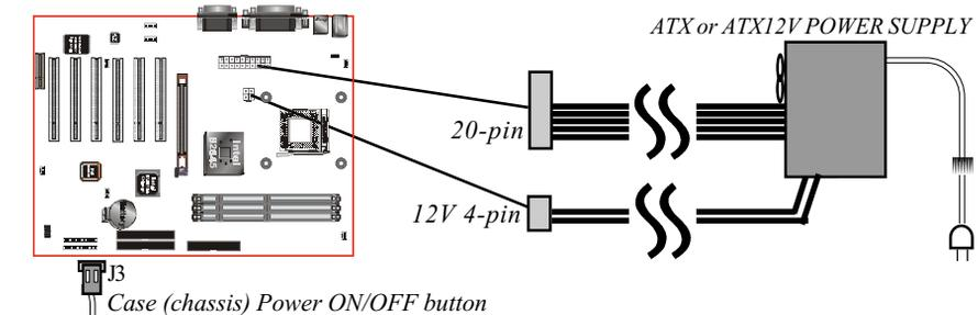
Figure 4: Simple ATX or ATX12V Power ON/OFF Controller
