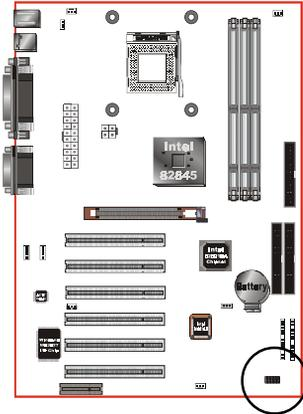
**USBCON1:** USB port header pins for share with two USB ports.
