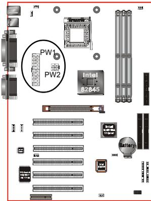
**PW1:** ATX or ATX12V Power Connector
