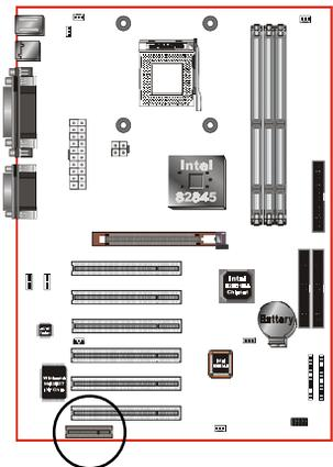
**CNR Conn.:** The board supports one CNR connector to provide a Modem Code (MC) or Phone-line base networking and 10/100 Ethernet base networking configuration.
