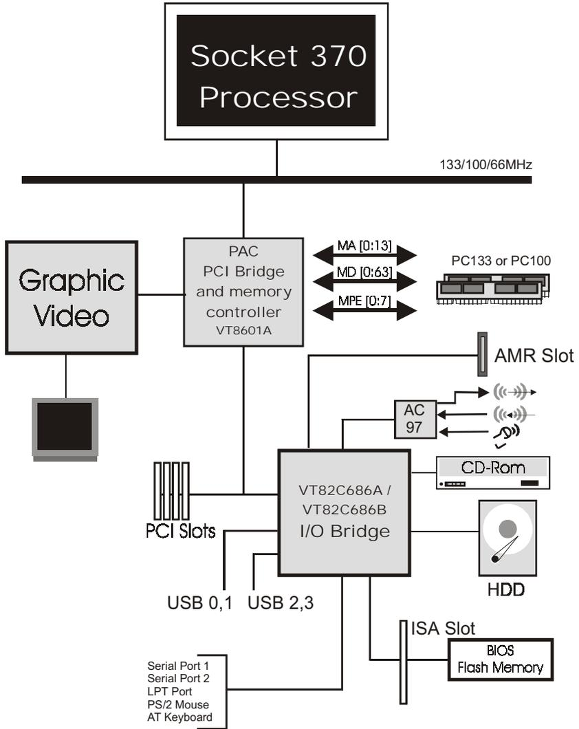
Figure 3: System Block Diagram
