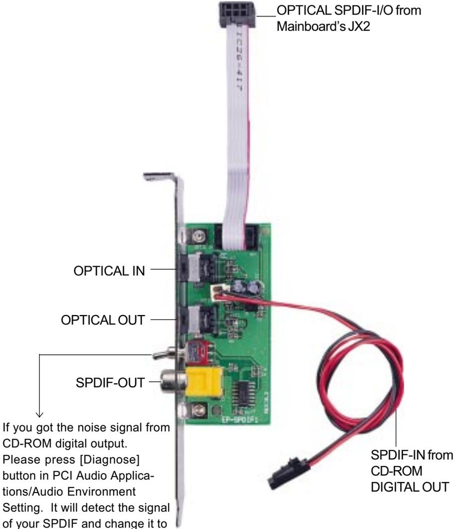
If you got the noise signal from CD-ROM digital output. Please press [Diagnose] button in PCI Audio Applications/Audio Environment Setting. It will detect the signal of your SPDIF and change it to be the correct format. If still can't match the format then switch the DIP switch to correct format.
