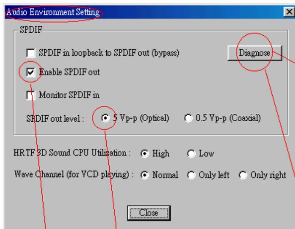
If you got the noise signal from CD digital output. Please press [Diagnose] button. It will detect the signal of your SPDIF and change it to be the correct format.
