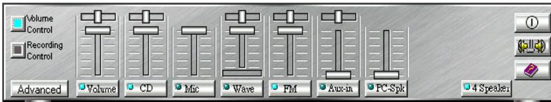
Mixer panel while the four speakers mode is enabled.
