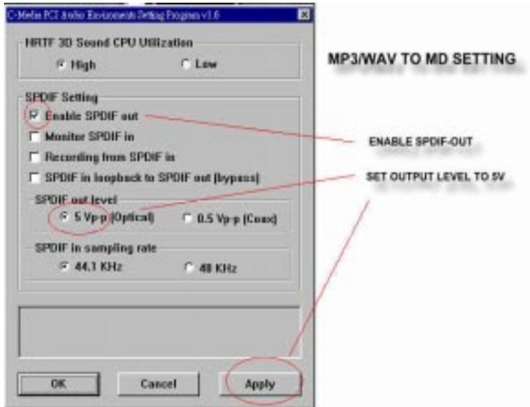
When all the procedures have been completed, there will be an infrared signal coming from the SPDIF/OUT of the optical fiber of the sound card.
