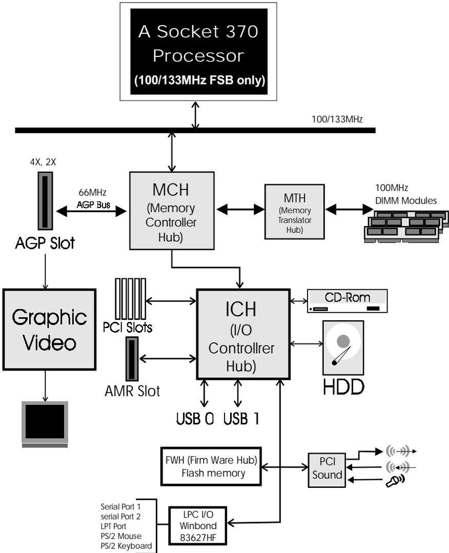
Figure 6: System Block Diagram
