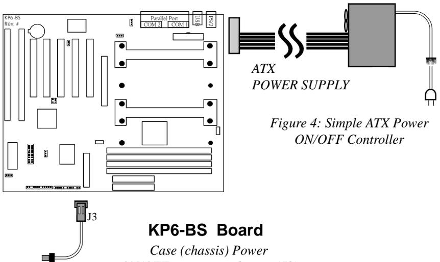
Figure 4: Simple ATX Power
