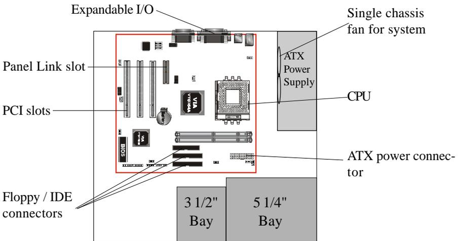
Figure 2: Summary of Micro ATX chassis features
