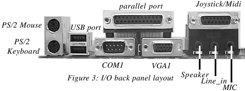
Figure 3: I/O back panel layout
