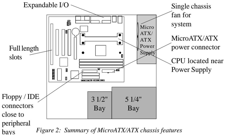
Figure 2: Summary of MicroATX/ATX chassis features
