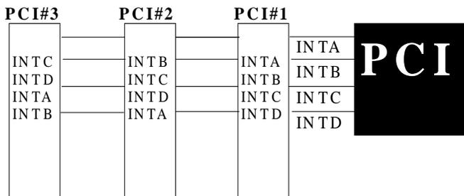
**Figure 7: The Combination of PCI INT#lines**
