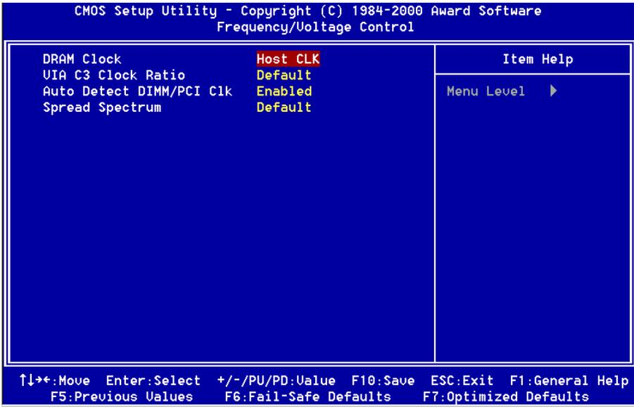
**DRAM Clock:** This setting controls the memory clock. The default is Host Clock.
