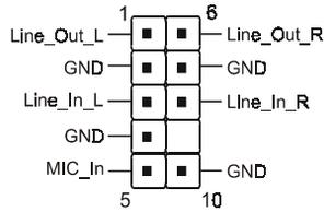
**Note:** Either Front Panel Audio or onboard rear audio could be used at one time.
